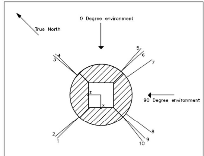
Fig. 18. Prototype spar mooring configuration.
