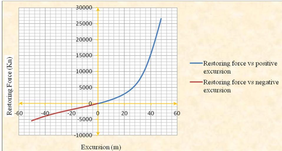
Fig. 5. Quasi-static simulation: restoring force vs. horizontal excursion.
