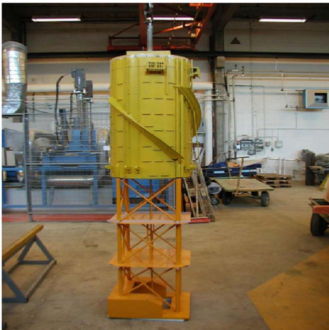
Fig. 17. A typical truss spar model at FORCE Technology.
