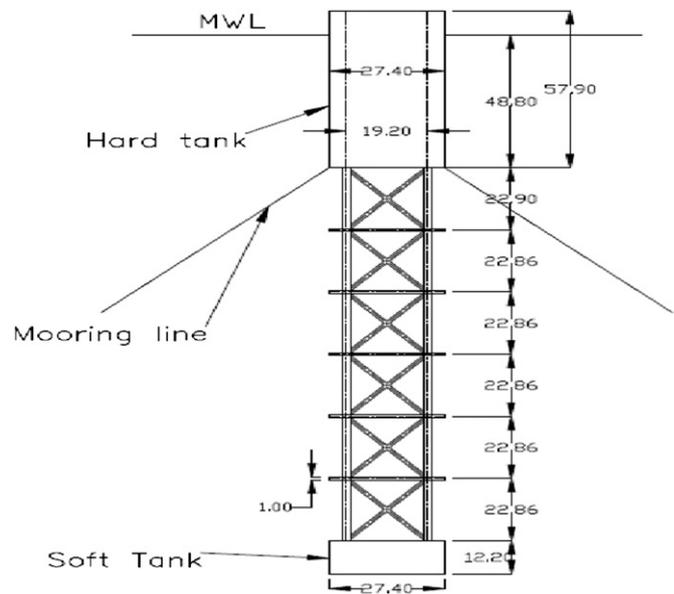
Fig. 4. Overall spar configuration (all dimensions are in m).
