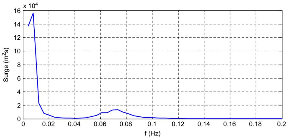
Fig. 6. Surge spectra: mean position (MP)+structure displacement (SD)+drag force (DF).
