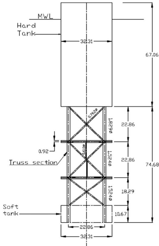
Fig. 16. Overall configuration of a typical truss spar platform (all dimensions are in m).
