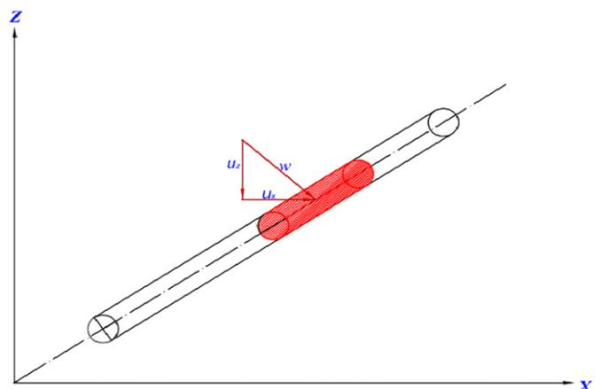
Fig. 2. Wave kinematics components on a segment on inclined cylinder.
