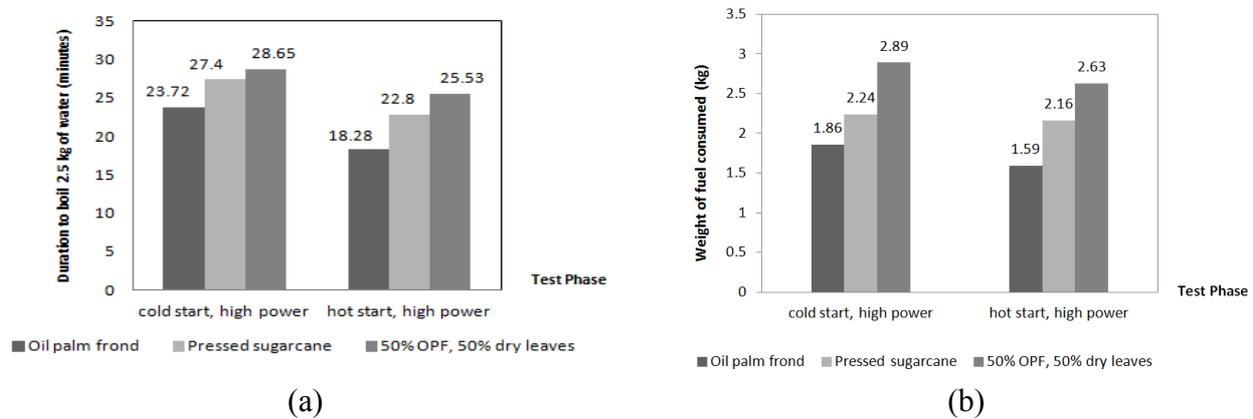
Fig.4: Cookstove performance in boiling 2.5 kg of water; (a) time duration, and (b) weight of fuel consumed
