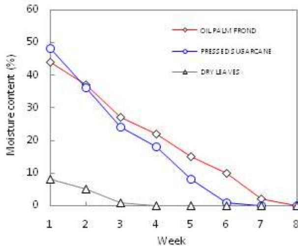
Fig.2:Variation of moisture content with time for different biomass materials
