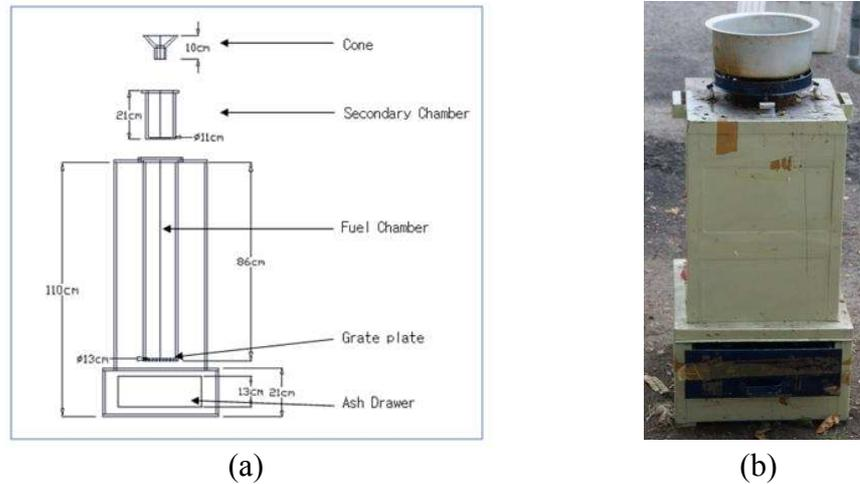
Fig. 3: Chemaco gasifier based cookstove: (a) schematic and (b) photograph
