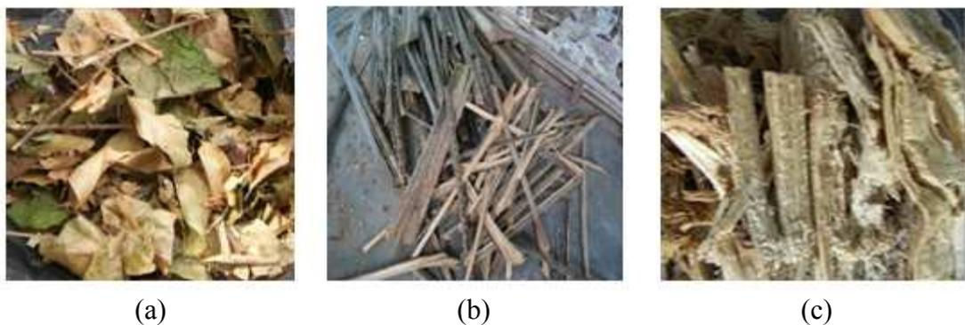
Fig.1:Raw biomass samples: (a) dry leaves, (b) oil palm fronds, and (c) pressed sugarcane
