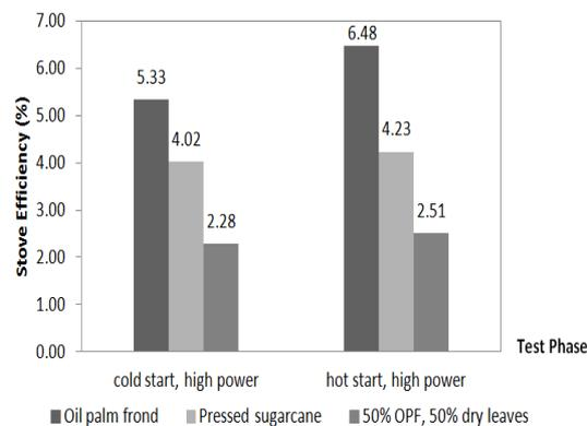
Fig. 5: Stove efficiency for different biomass and tests
