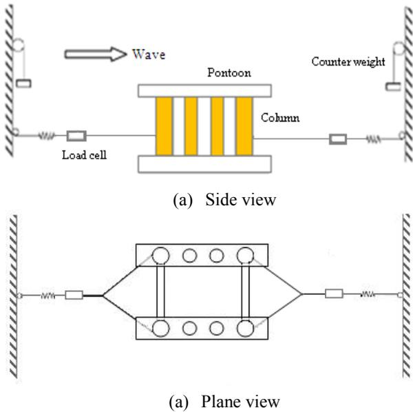
**Figure 1: Layout of model test**
