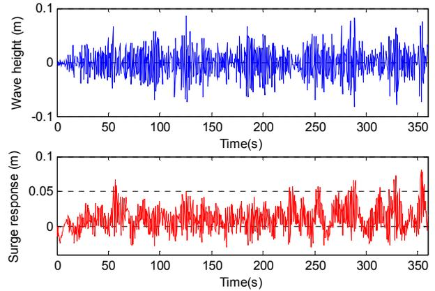
**Figure 2: Filtered wave height and surge response of IRW-1**
