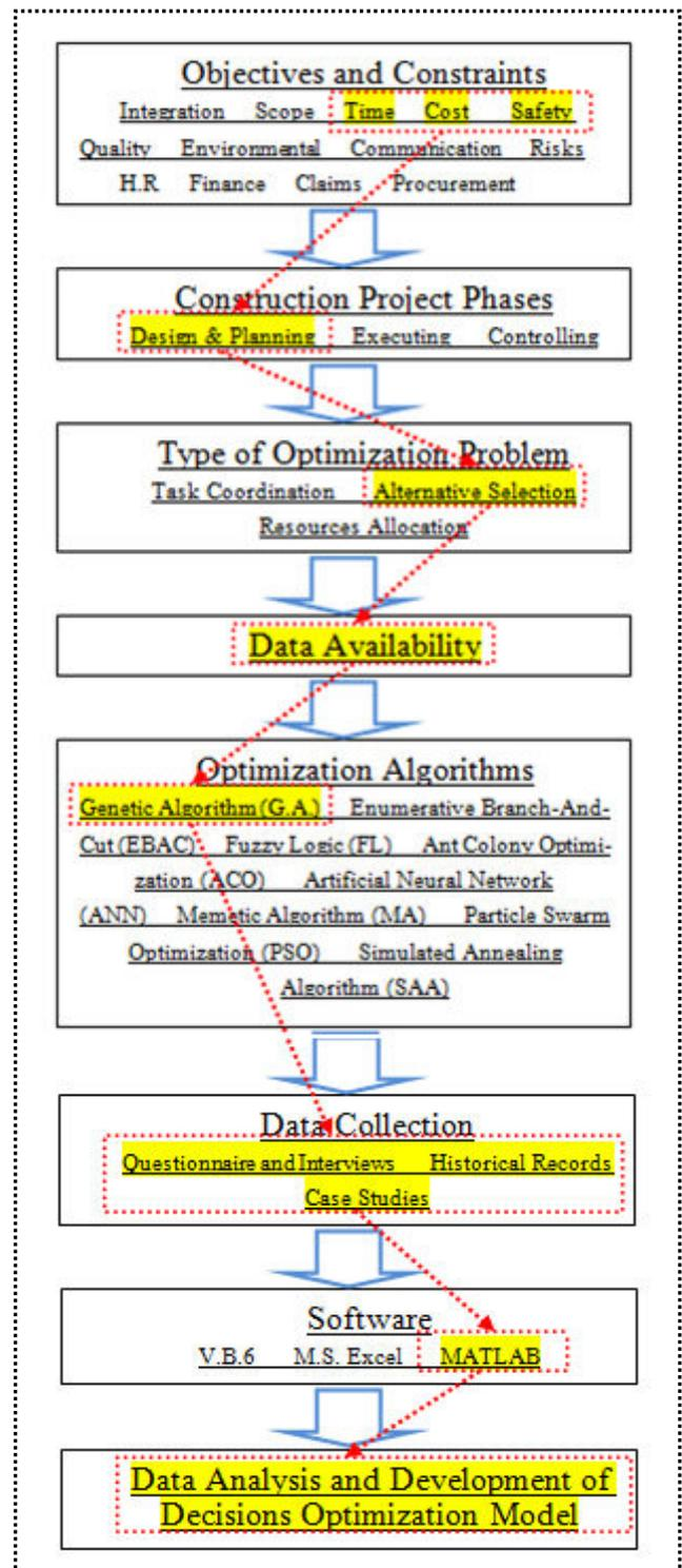
Fig(4): Flow chart for using optimization algorithms for developing decision making framework in construction management.
