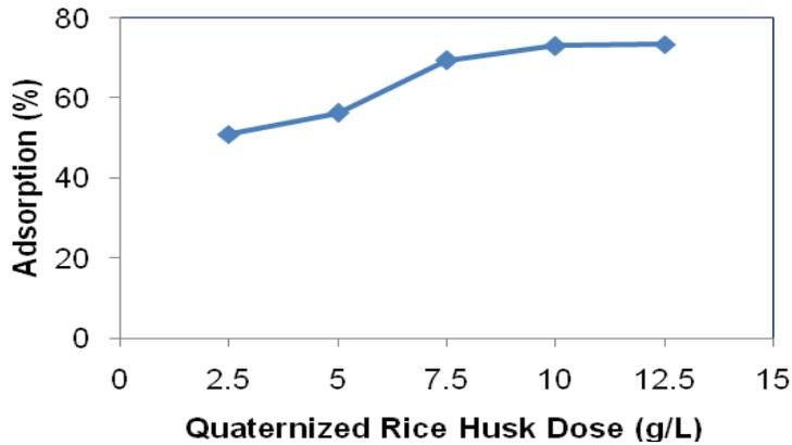
**Figure 3:** Effect of quarternized dose on adsorption.
