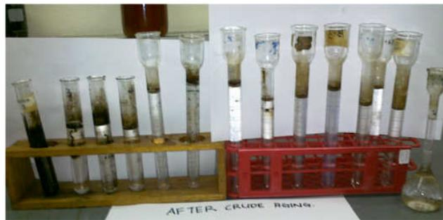
Figure 17 - Crude and brine were collected in test tubes at the outlet of core floods system after crude aging and flushing with brine
