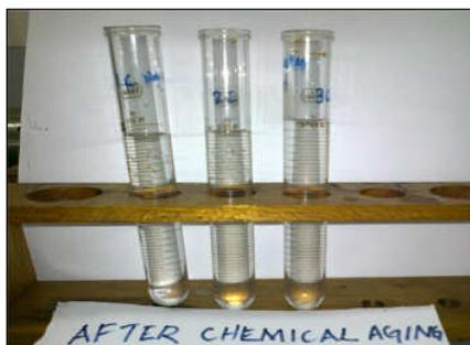
**Figure 12 - Brine collected after wax inhibitor was aging overnight**
