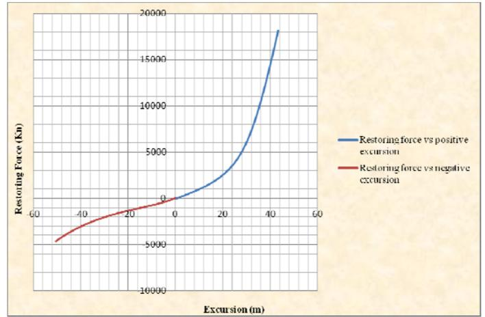
b) Surge static offset simulation for the additional mooring lines.
