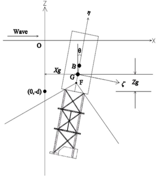
Fig. 1 Three DOF Surge-heave-pitch Model of the Spar
