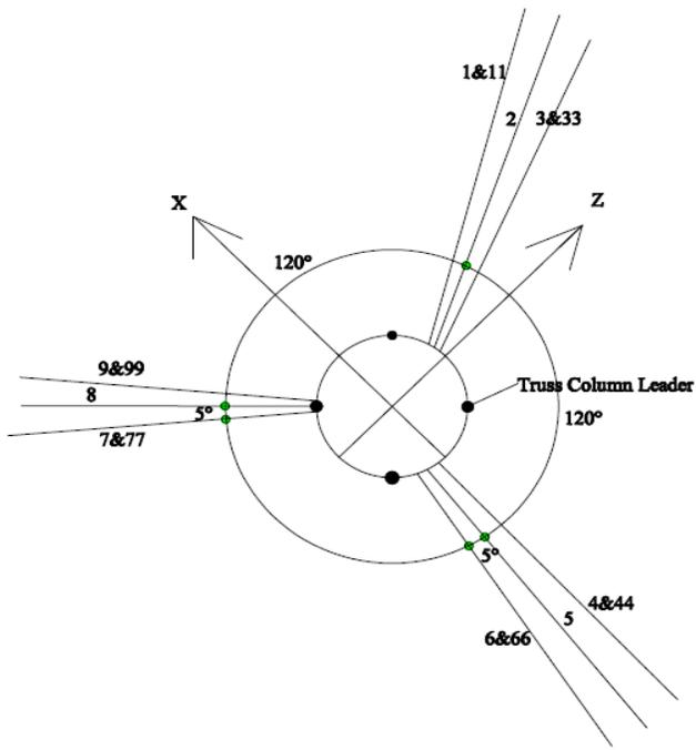
Fig. 3. Mooring lines arrangement
