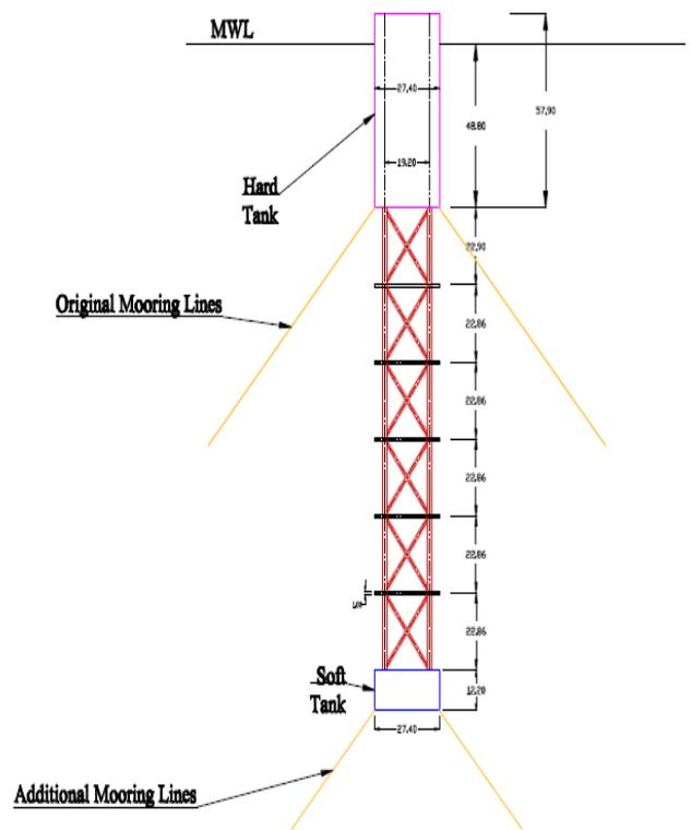
Fig. 2. Overall spar configuration with the additional mooring lines
