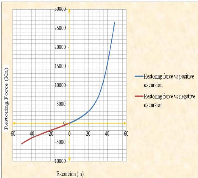
a) Surge static offset simulation for the original mooring lines..
