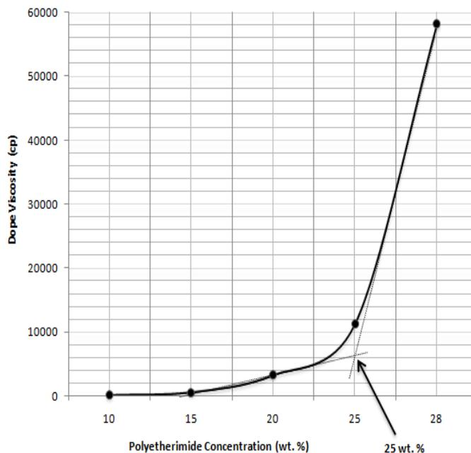
**Figure 1:** Critical dope viscosity for PEI/NMP solution.
