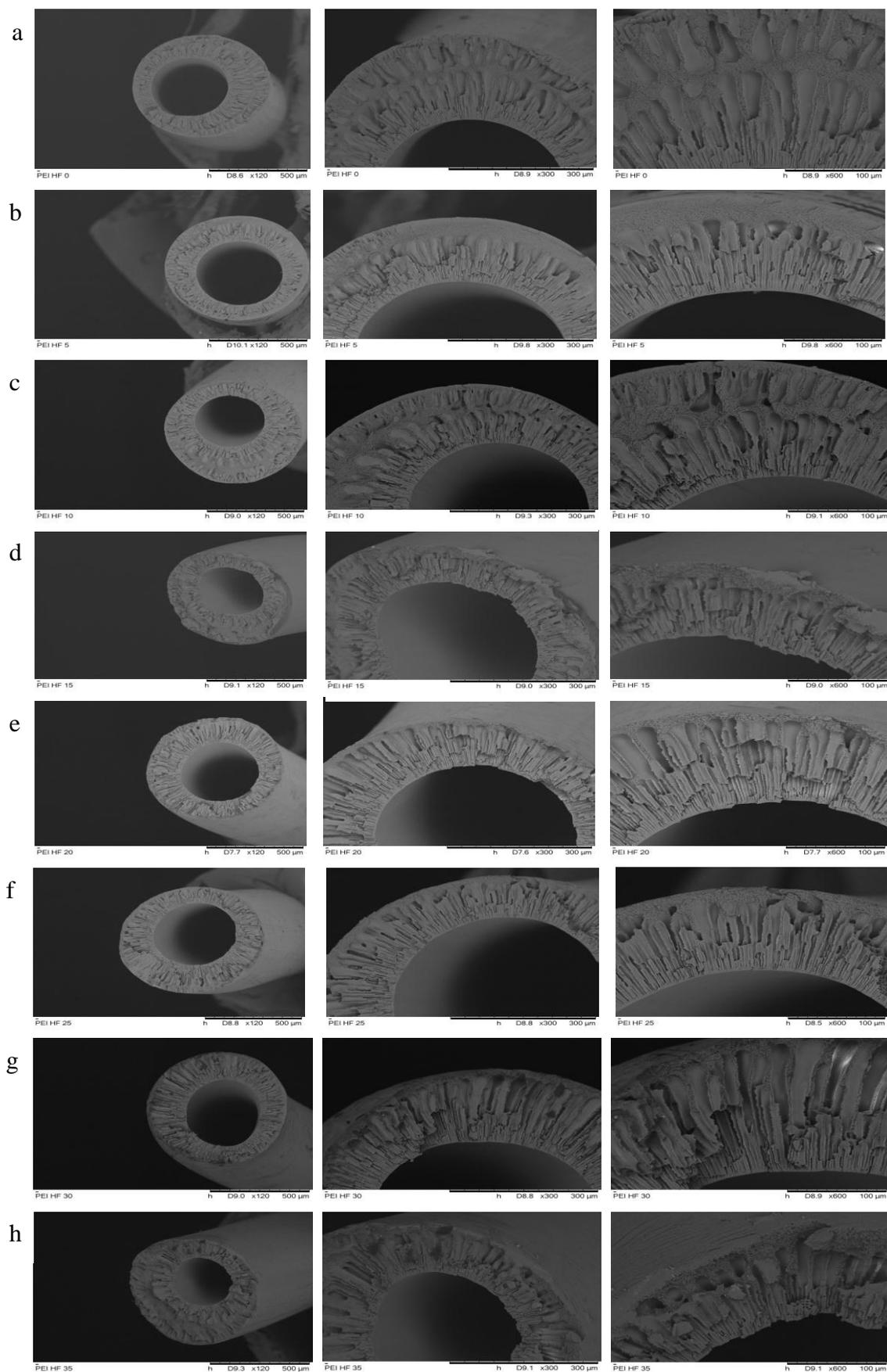
**Figure 2.** SEM images of PEI/NMP hollow fibre membranes (PEI, 25 wt.%), where rows a, b, c, d, e, f, g, h are representing air gaps in cm of 0, 5, 10, 15, 20, 25, 30 and 35 respectively.
