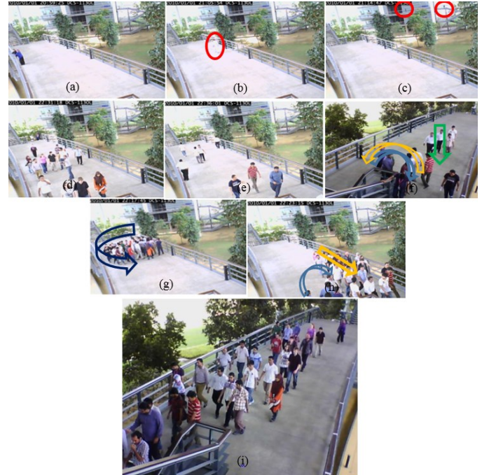
Fig. 6. Sample frames resembling various background modeling challenges; (a) to (c) are for single object detection for challenges of sleeping foreground objects, camouflage, depth object detection and gradual illumination. Sample frames (d) to (f) resemble random motion of sparse crowds, heavy illumination variance and different motion scenarios. Frames (g) to (i) are sample frames of dense crowd, performing arch ring, bottleneck and lane motion scenarios under heavy illumination variance in the background of multiple camera views.
