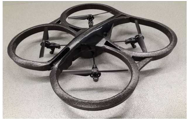
Fig. 5. Parrot AR.Drone (UAV used in the experiment)
