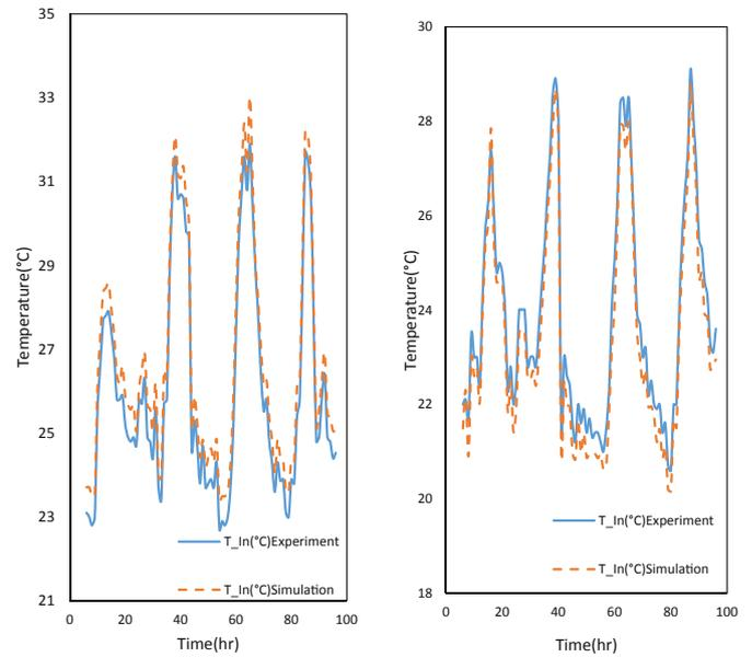
Fig. 11. Comparison of experimental and simulation data for indoor air temperature of test room when TE-AD system operated at 5A and 6A.
