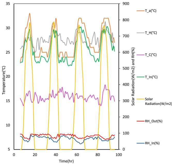
Fig. 8. Variation of indoor and outdoor climatic conditions of test room with time, when TE-AD system operated at 7A.
