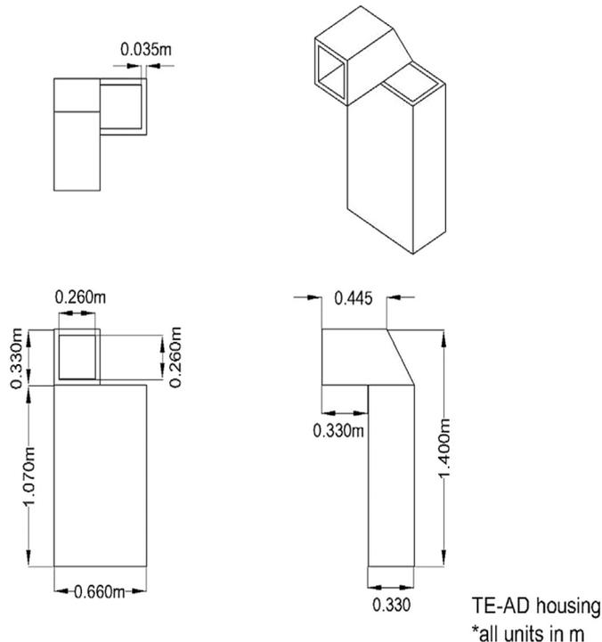
Fig. 3. Dimensional details of TE-AD.
