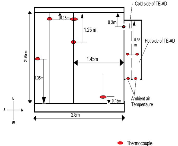
Fig. 4. Arrangement of thermocouple for temperature recording.
