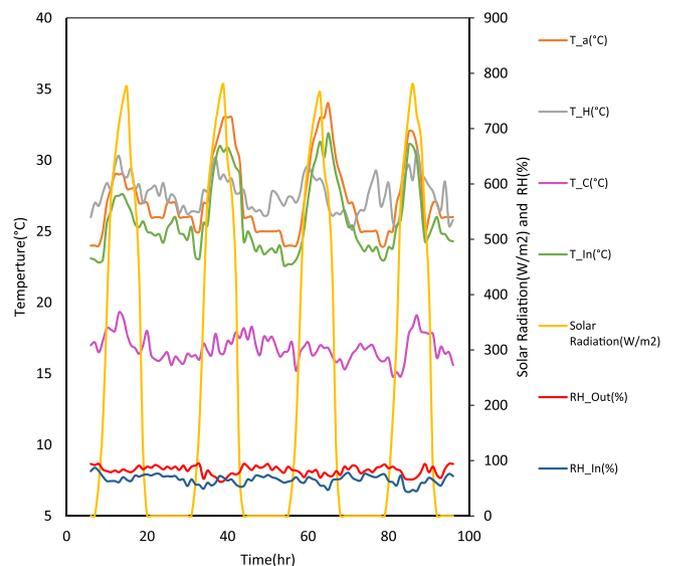
**Fig. 6.** Variation of indoor and outdoor climatic conditions of test room with time, when TE-AD system operated at 5A.
