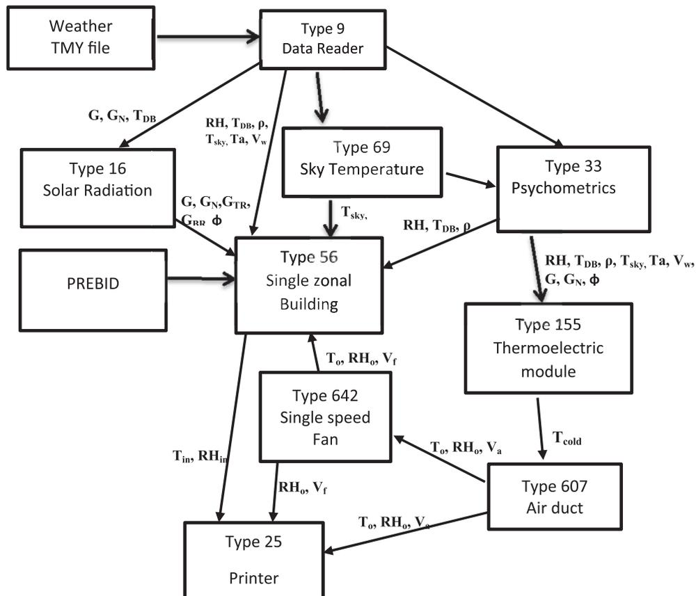
Fig. 5. TRNSYS information flow diagram.
