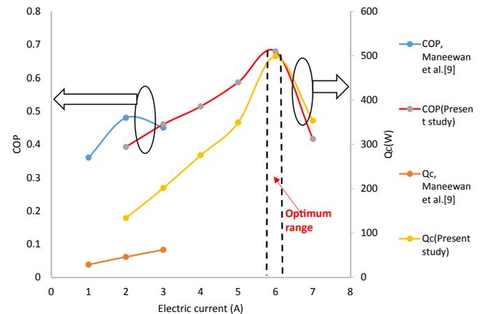
Fig. 9. Comparison of COP and cooling power of TE-AD system with previous study.
