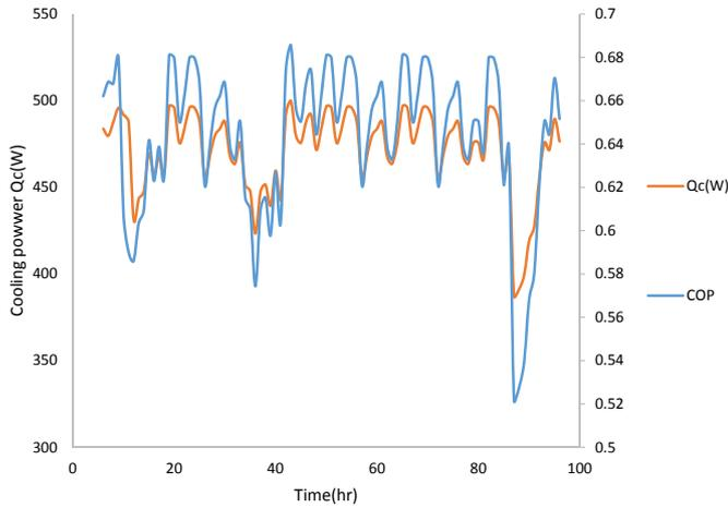
Fig. 10. Variation of COP and cooling capacity of test room with time, when TE-AD system operated at 6A.
