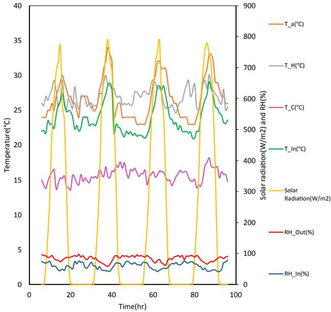
Fig. 7. Variation of indoor and outdoor climatic conditions of test room with time, when TE-AD system operated at 6A.
