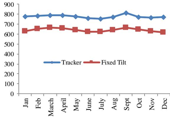
Figure 20. Graphical representation of monthly solar insolation available to fixed tilt solar system and sun-tracked solar system
