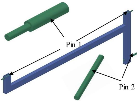
Figure 8. Diagram of the supporting pins
