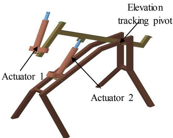
Figure 10. Actuators and the hinge mechanism
