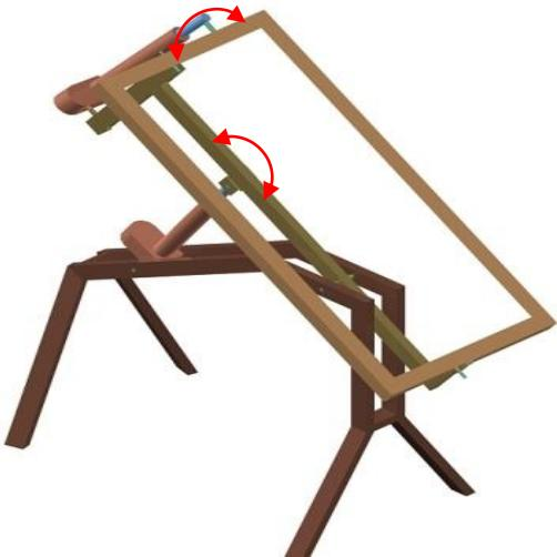
Figure 14. Illustration of azimuth and elevation tracking directions
