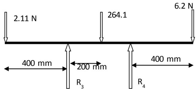
Figure 11. Free body diagram of the forces acting at  $R_3$  and  $R_4$
