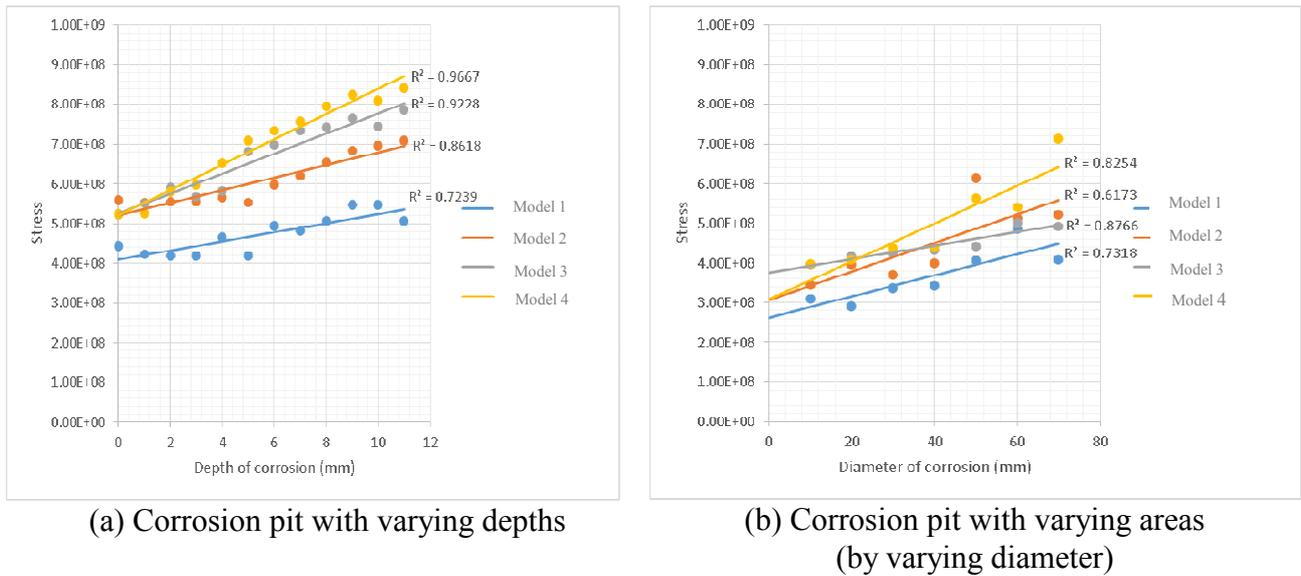
Figure 4. Stress distributions obtained for different corrosion scenarios
