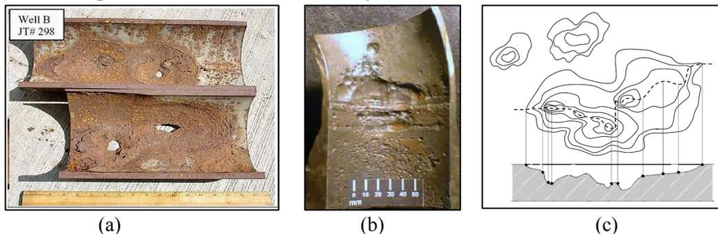
Figure 1. Examples and sketch of pipeline failures due to internal corrosions
