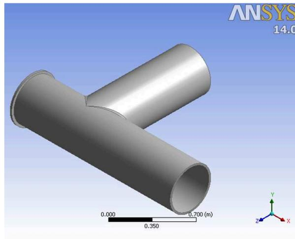
(c) Unbarred full-bored pipe bend near dead end (Model 3)
