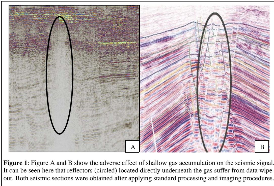
**Figure 1:** Figure A and B show the adverse effect of shallow gas accumulation on the seismic signal. It can be seen here that reflectors (circled) located directly underneath the gas suffer from data wipe-out. Both seismic sections were obtained after applying standard processing and imaging procedures.
