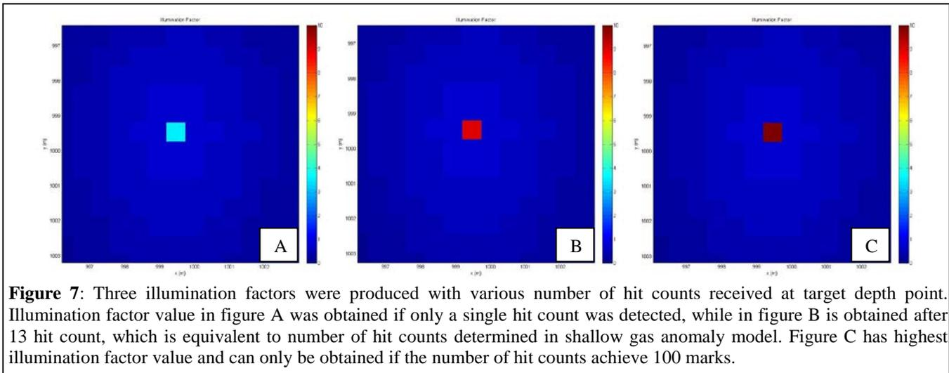
**Figure 7:** Three illumination factors were produced with various number of hit counts received at target depth point. Illumination factor value in figure A was obtained if only a single hit count was detected, while in figure B is obtained after 13 hit count, which is equivalent to number of hit counts determined in shallow gas anomaly model. Figure C has highest illumination factor value and can only be obtained if the number of hit counts achieve 100 marks.
