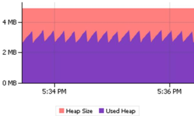
Fig. 7. Saw tooth utilization of heap memory in task 1.
