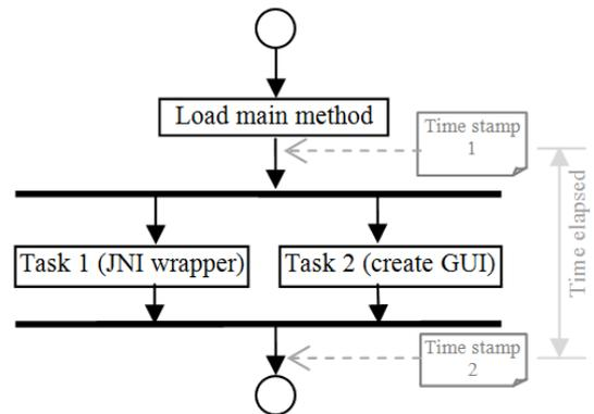
Fig. 6. Measuring elapsed time in concurrent tasks.
