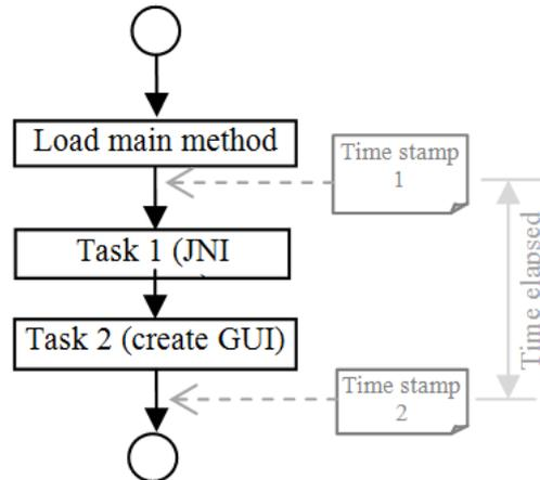
Fig. 5. Measuring elapsed time in sequential tasks.
