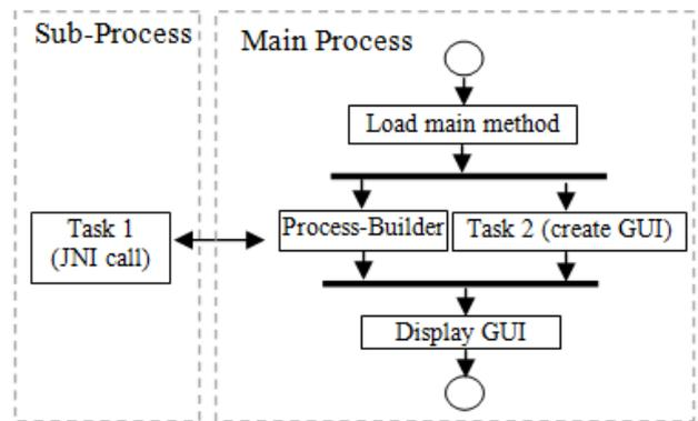
Fig. 11. Proposed multi-processing using Java ProcessBuilder.
