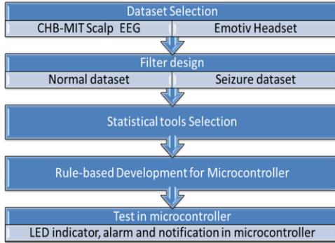
Figure 2. Flowchart of the Wearable Computing System for the Seizure Detection.
