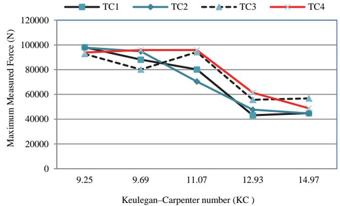
Fig. 6. Comparison showing the variation of maximum hydrodynamic forces on a tubular cylinder due to the effects of cylinder proximity presented versus  $KC$  number
