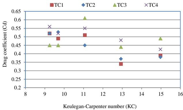
Fig. 7. Comparison showing the variation of drag coefficients for a tubular cylinder with outer diameter  $D_o = 1.87$  m, with different test configurations as a function of KC number
