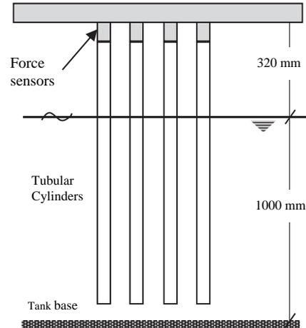
Fig. 1. Details of the model setup in the wave basin
