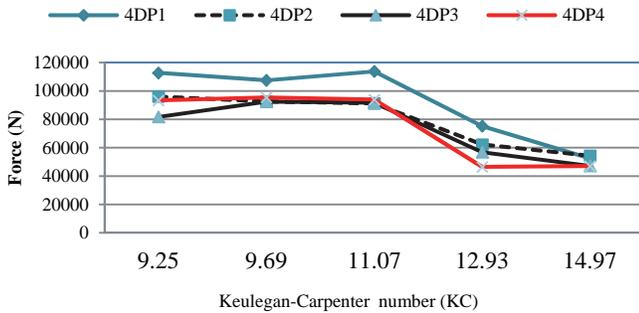
Fig. 10. Comparison of hydrodynamic forces for array of tubular cylinders, with center to center spacing  $S_x = 4D$ .
