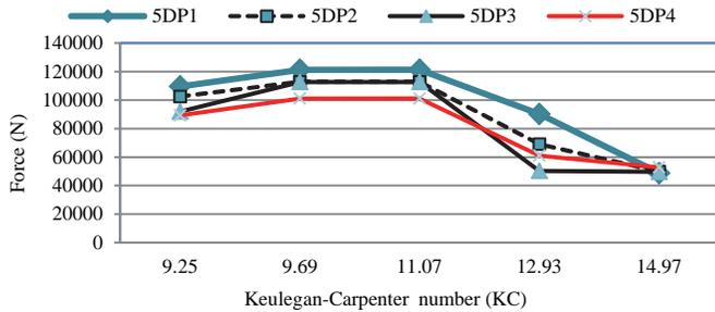
Fig. 11. Comparison of hydrodynamic forces for array of tubular cylinders, with center to center spacing  $S_x = 5D$ .
