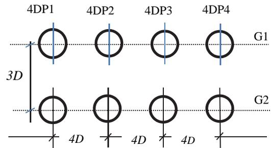
Fig. 4. Model configurations for rectangular arrays, with center to center spacing  $S_x = 4D$
