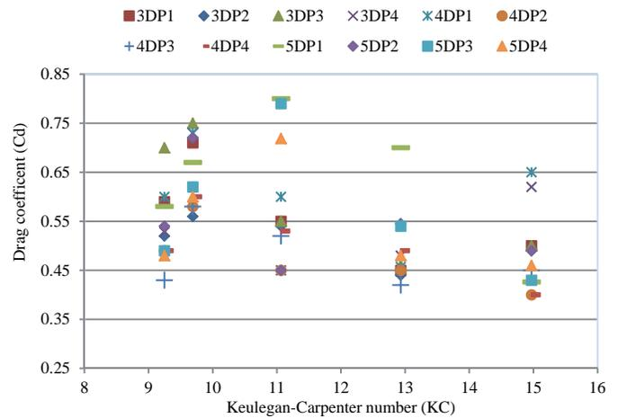
Fig. 14. Comparison of drag coefficients for array of cylinders, with different center to center spacing  $S_x = 3D$ ,  $4D$ , and  $5D$  as a function of KC number
