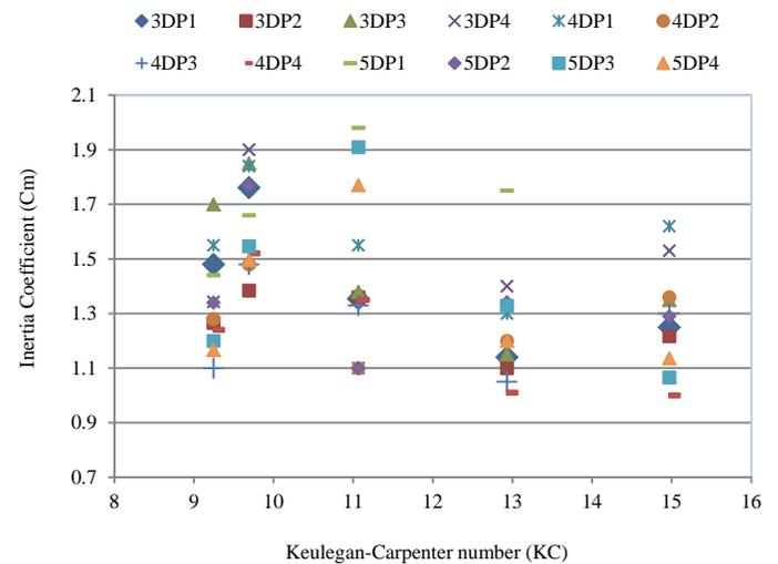
Fig. 15. Comparison of inertia coefficients for array of cylinders, with different center to center spacing  $S_x = 3D$ ,  $4D$ , and  $5D$  as a function of KC number.
