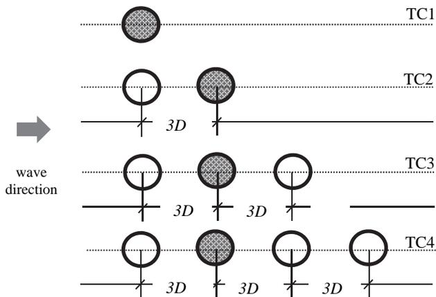
Fig. 2. Different test configurations for array of tubular cylinders in tandem arrangement
