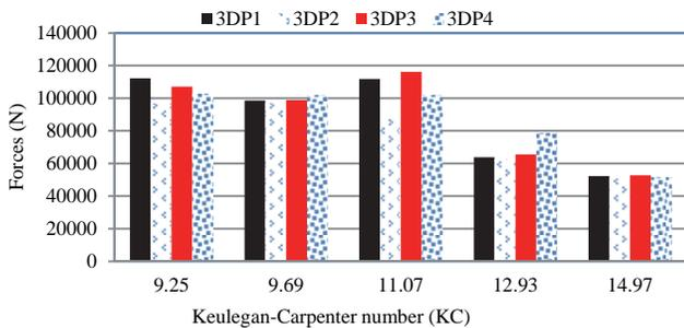
Fig. 12. Comparison of hydrodynamic forces for four tubular cylinders in tandem arrangement, with center to center spacing  $S_x = 3D$ , for different KC numbers
