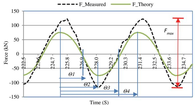
Fig. 13. Schematic diagram showing the measured and theoretically estimated hydrodynamic forces and the phase angles adopted for determination of  $C_m$  and  $C_d$  values
