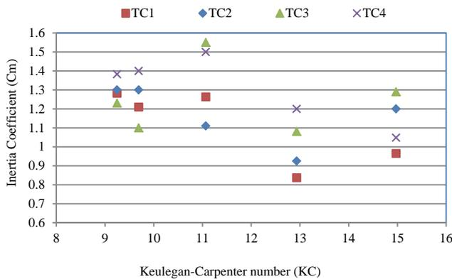
Fig. 8. Comparison showing the variation of inertia coefficients for a tubular cylinder with outer diameter  $D_o = 1.87$  m, with different test configurations as a function of KC number
