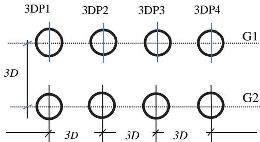
Fig. 3. Model configurations for rectangular arrays, with center to center spacing  $S_x = 3D$
