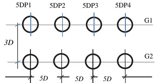
Fig. 5. Model configurations for rectangular arrays, with center to center spacing  $S_x = 5D$
