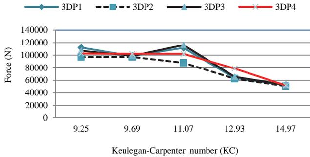
Fig. 9. Comparison of hydrodynamic forces for array of tubular cylinders, with center to center spacing  $S_x = 3D$ .
