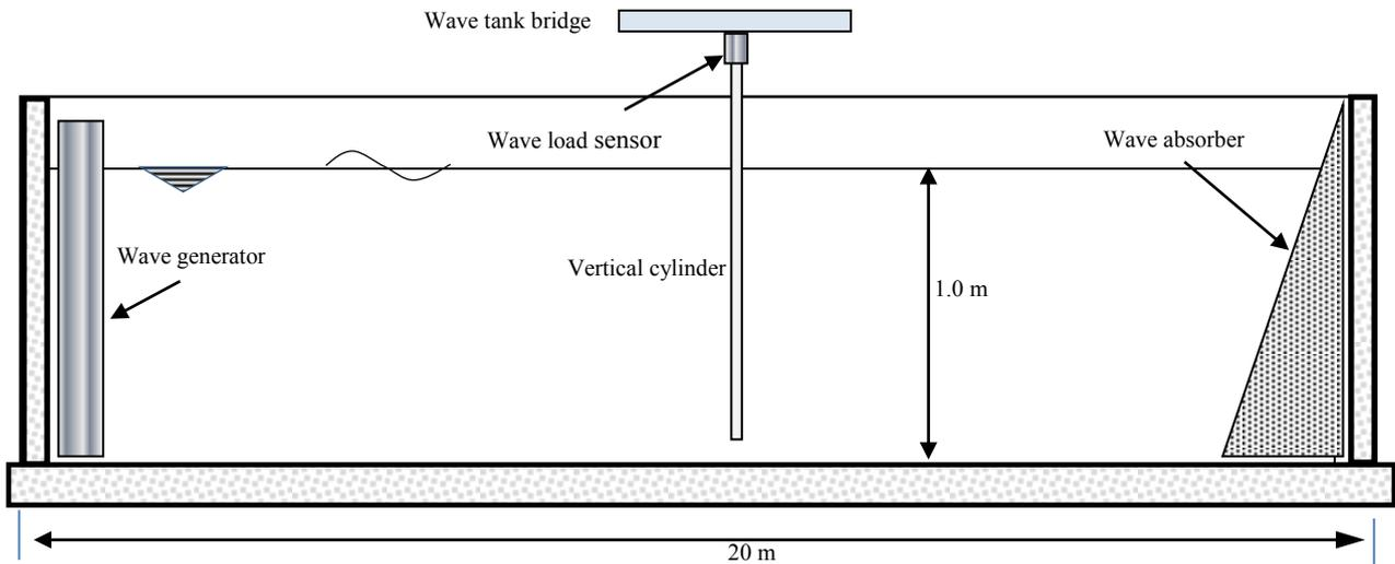
Fig. 2. Cross sectional elevation of wave tank with the model specimen details
