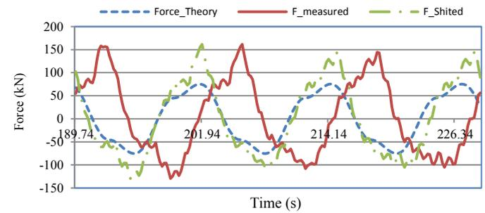
Fig. 8. Comparison of experimental and numerical hydrodynamic forces for 1.36 m diameter cylinder subjected to regular waves with  $H_{max}=8$  m and frequency,  $f = 0.079$  Hz
