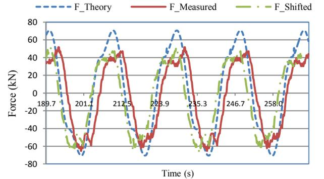
Fig. 4. Comparison of experimental and numerical hydrodynamic forces for 1.68 m diameter cylinder subjected to regular waves with  $H_{max} = 8$  m, and frequency,  $f = 0.052$  Hz
