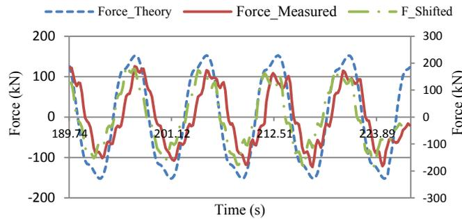
Fig. 6. Comparison of experimental and numerical hydrodynamic forces for 1.68 m diameter cylinder subjected to regular waves with  $H_{max}=8$  m, and frequency,  $f = 0.127$  Hz
