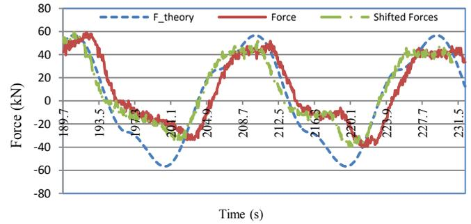
Fig. 7. Comparison of experimental and numerical hydrodynamic forces for 1.36 m diameter cylinder subjected to regular waves with  $H_{max}=8$  m, and frequency,  $f = 0.052$  Hz
