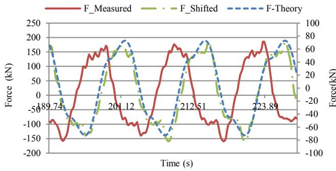
Fig. 5. Comparison of experimental and numerical hydrodynamic forces for 1.68 m diameter cylinder subjected to regular waves with  $H_{max}=8$  m, and frequency,  $f = 0.079$  Hz
