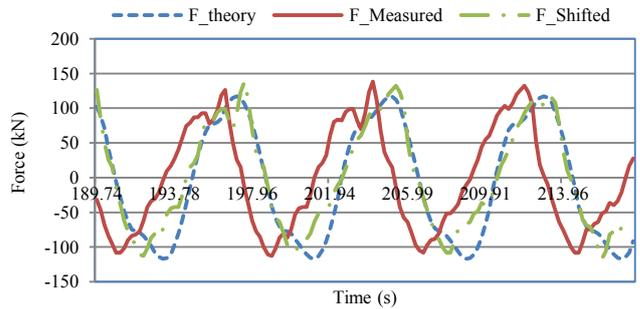
Fig. 9. Comparison of experimental and numerical hydrodynamic forces for 1.36 m diameter cylinder subjected to regular waves with  $H_{max}=8$  m and frequency,  $f = 0.127$  Hz
