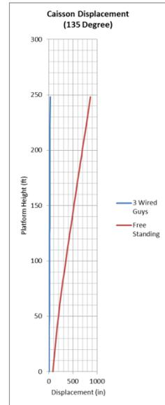
Figure 8: Caisson Displacement at 135° Direction
