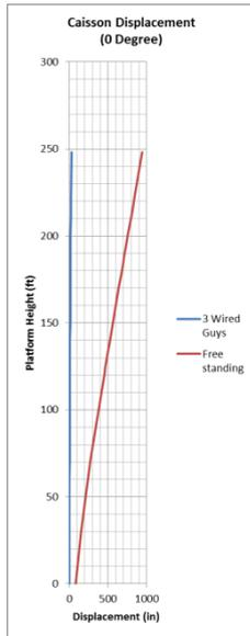
Figure 5: Caisson Displacement at 0° Direction
