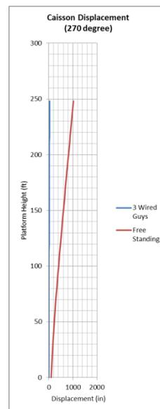
Figure 11: Caisson Displacement at 270° Direction
