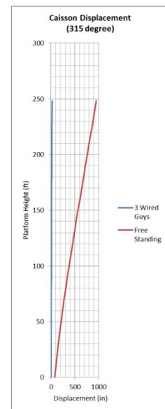
Figure 12: Caisson Displacement at 315° Direction
