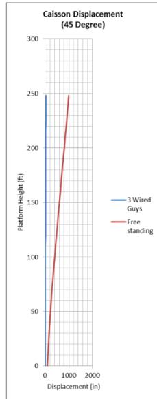
Figure 6: Caisson Displacement at 45° Direction
