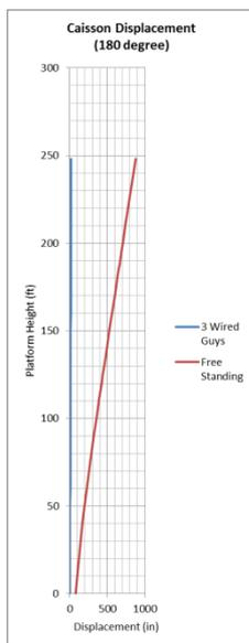
Figure 9: Caisson Displacement at 180° Direction
