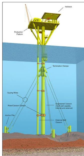
Figure 2: Typical designs for Tarpon system
