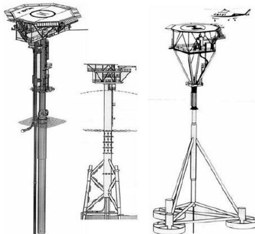
Figure 1: Typical monopod platforms used in shallow water
