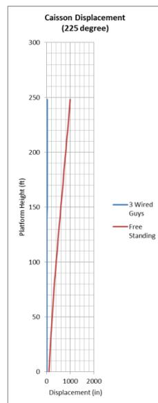
Figure 10: Caisson Displacement at 225° Direction
