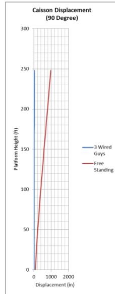
Figure 7: Caisson Displacement at 90° Direction
