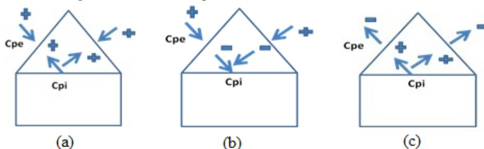
Figure 2: Cases of roof wind pressure on duopitch rectangular buildings
