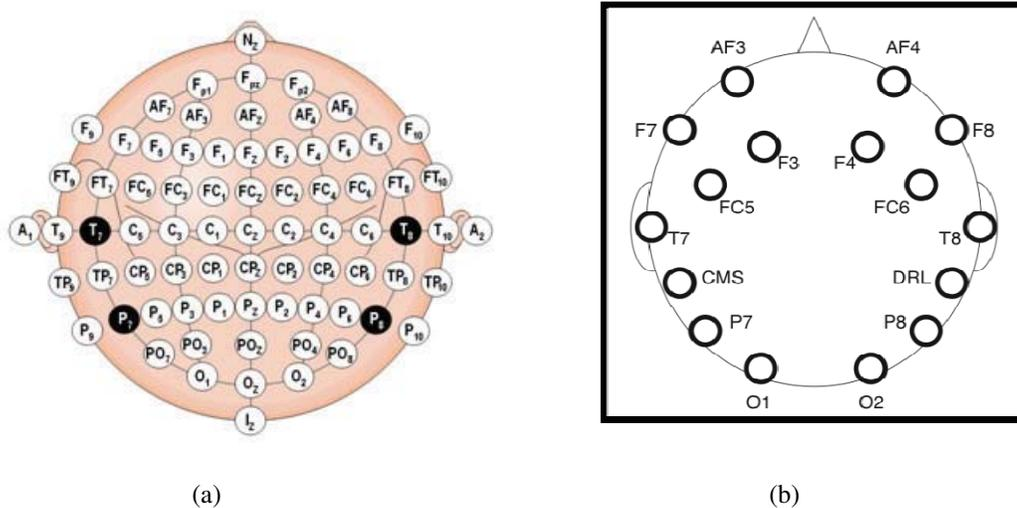
**FIGURE 1.** (a)The international 10-20 system or conventional electrode positioning, (b) Emotive EPOCH electrode positioning
