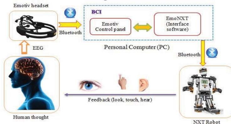
FIGURE 2. Block diagram of the proposed BCI System
