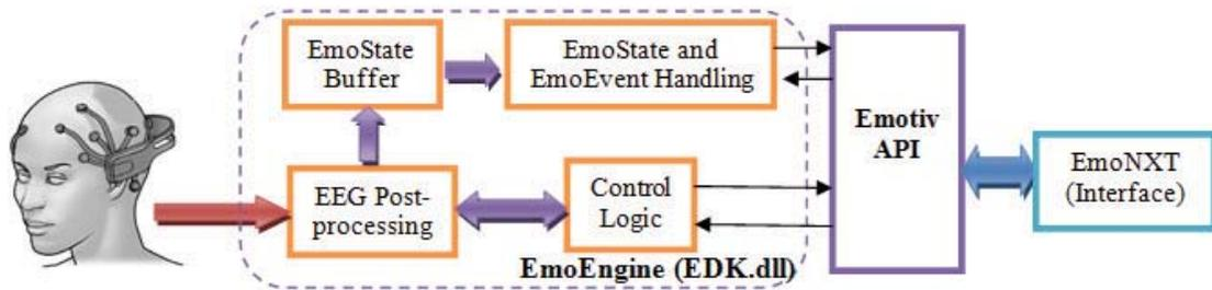
FIGURE 2. Block diagram of interface between EMOTIV and NXT robot
