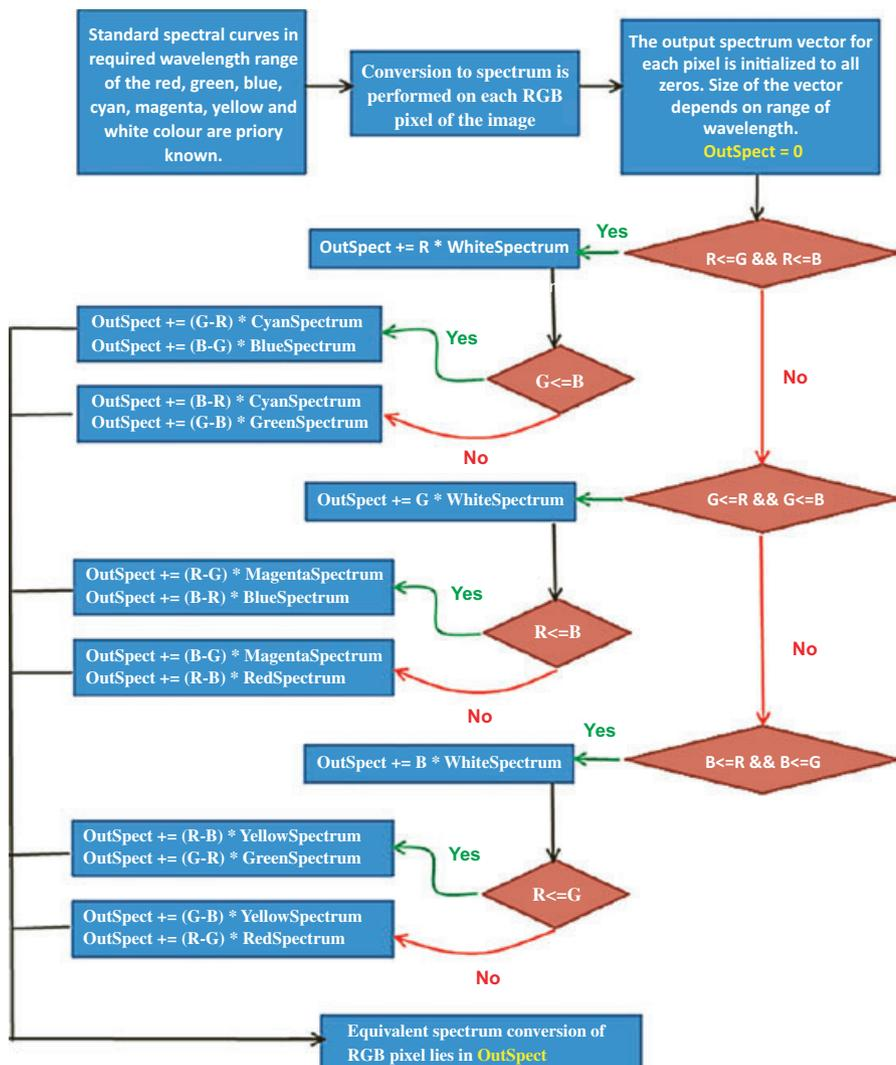
Fig. 3. Diagram of process flow of RGB to spectrum conversion.
