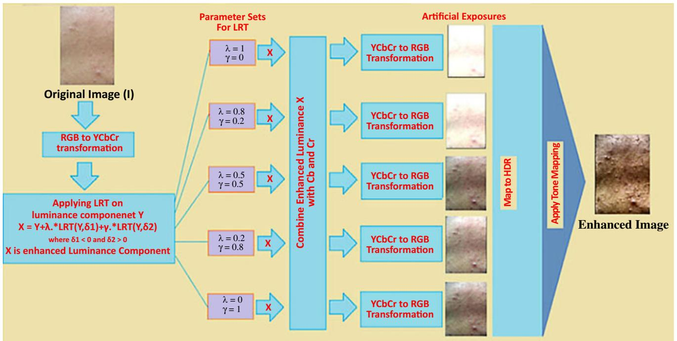
Fig. 2. Proposed contrast enhancement process flow diagram.
