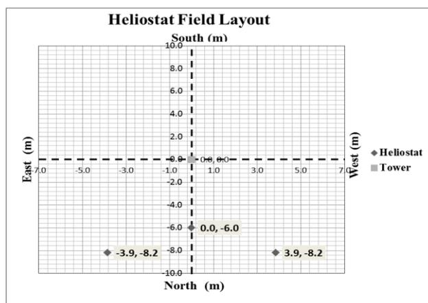
**Figure 2.** Final Field Layout for the 3 heliostat units.
