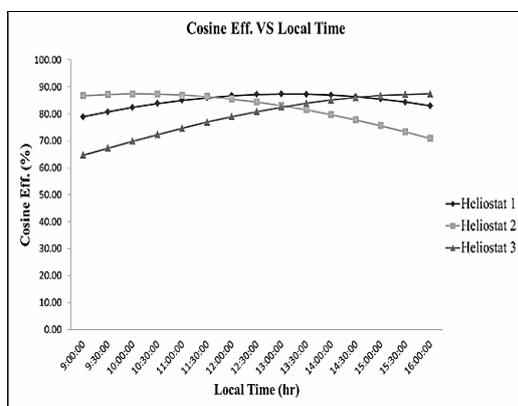
**Figure 3.** Cosine efficiency for heliostat 1, heliostat 2, and heliostat 3 at September 23.
