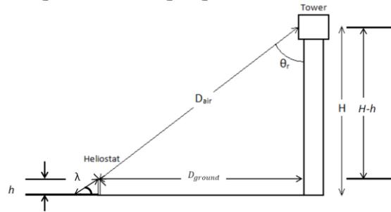
**Figure 1.** Tower and Heliostat trigonometry relationships.
