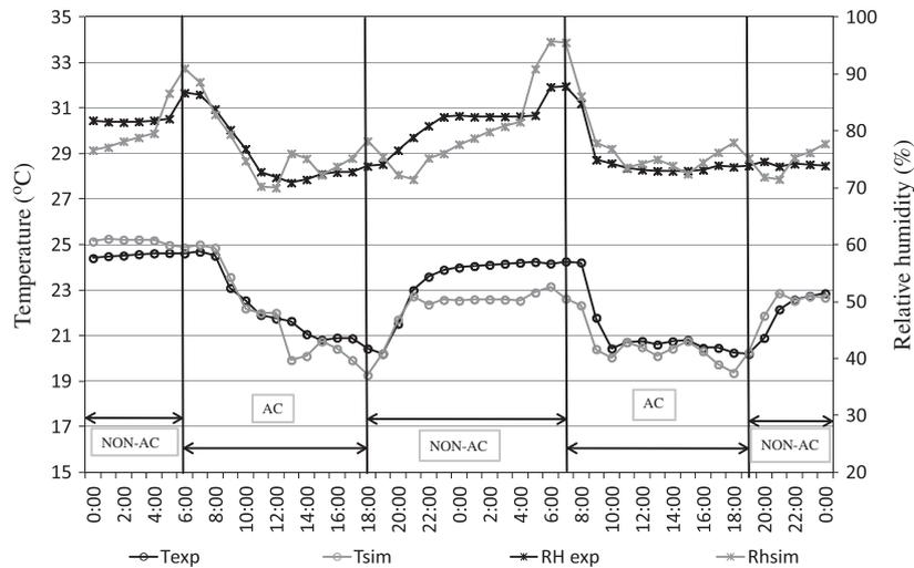
Fig. 7. Comparison of predicted and measured indoor temperature and relative humidity during weekdays.
