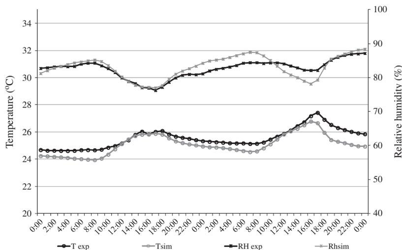
Fig. 6. Comparison of predicted and measured indoor temperature and relative humidity during weekends.
