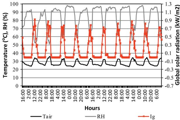
Fig. 5. Experimental measurements of outdoor conditions (ambient temperature, ambient relative humidity and global solar radiation) [35].
