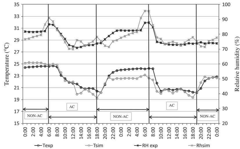
Fig. 7. Comparison of predicted and measured indoor temperature and relative humidity during weekdays.
