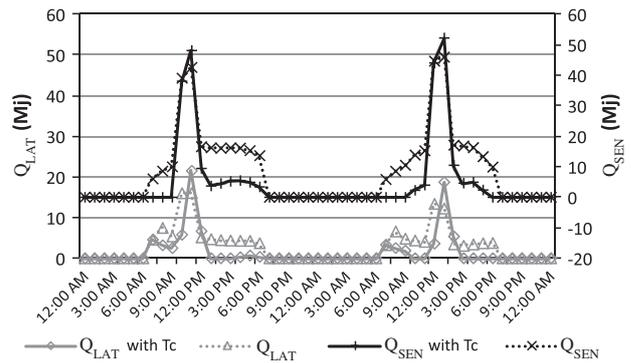
Fig. 10. Hourly cooling load characteristic in the workshop.
