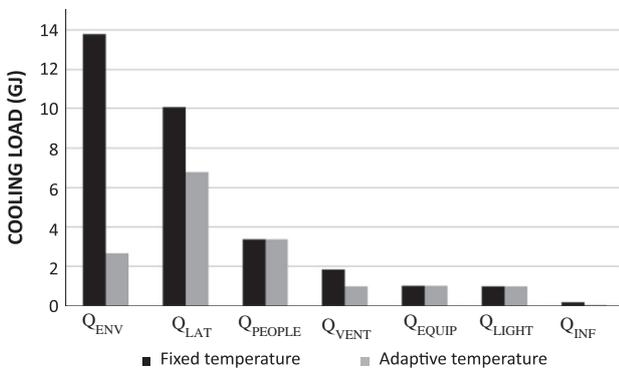
Fig. 13. Breakdown of yearly total cooling load in the classroom.
