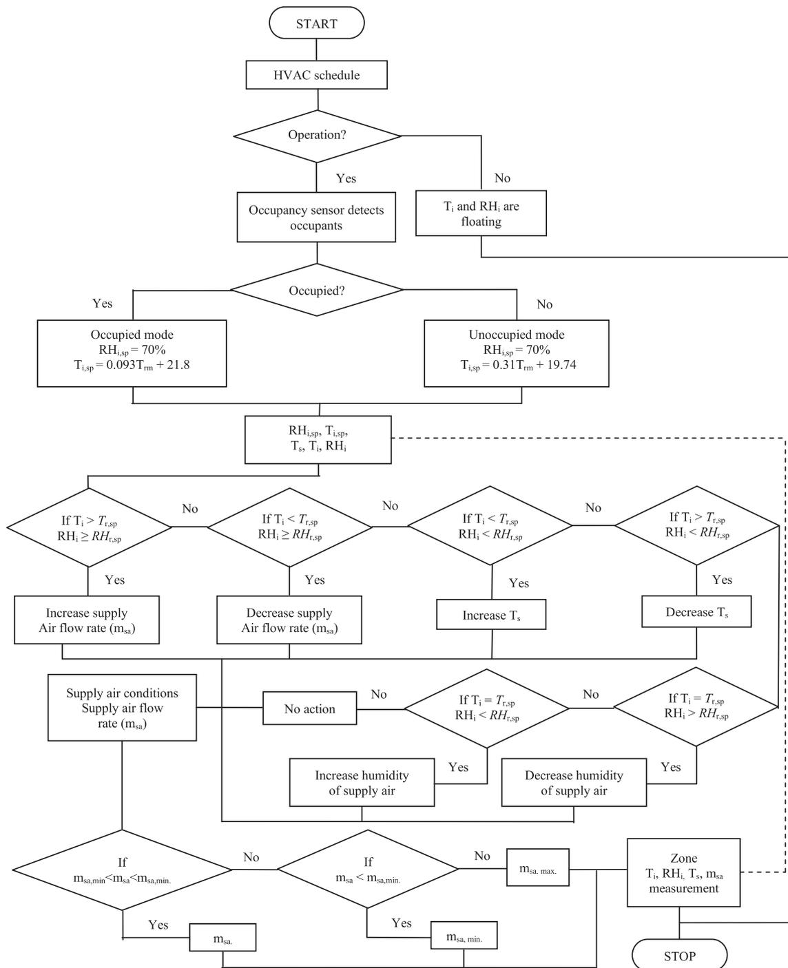
Fig. 8. Flow chart of proposed control system for the HVAC system.
