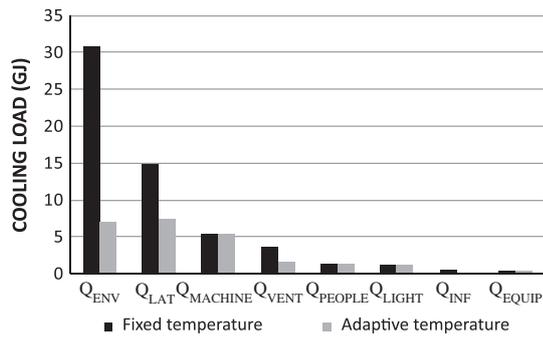
Fig. 11. Breakdown of yearly total cooling load in the workshop.
