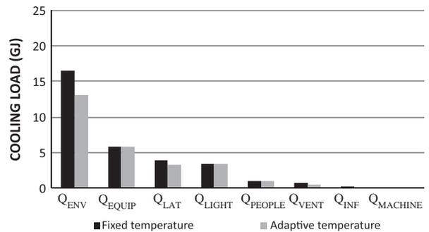
Fig. 15. Breakdown of yearly total cooling load in the office.
