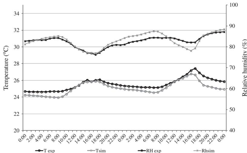
Fig. 6. Comparison of predicted and measured indoor temperature and relative humidity during weekends.
