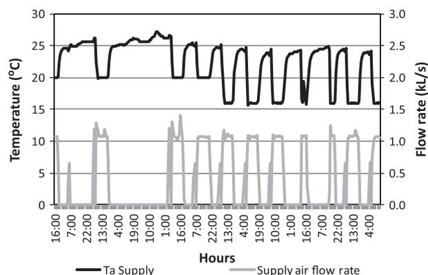
Fig. 4. Measurement of supply air temperature and flow rate entering the zone.
