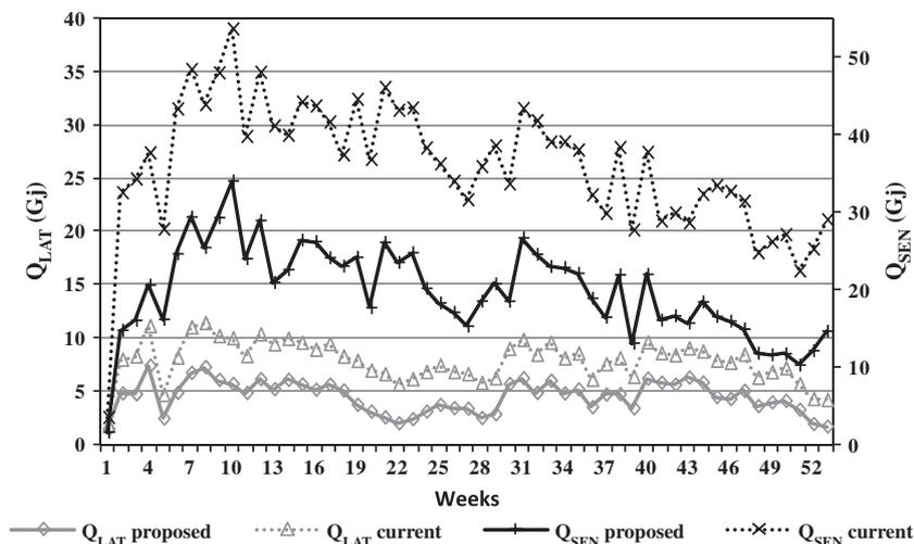
Fig. 9. Weekly average cooling load of the building.
