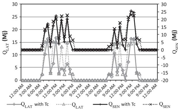
Fig. 12. Hourly cooling load characteristic in the classroom.
