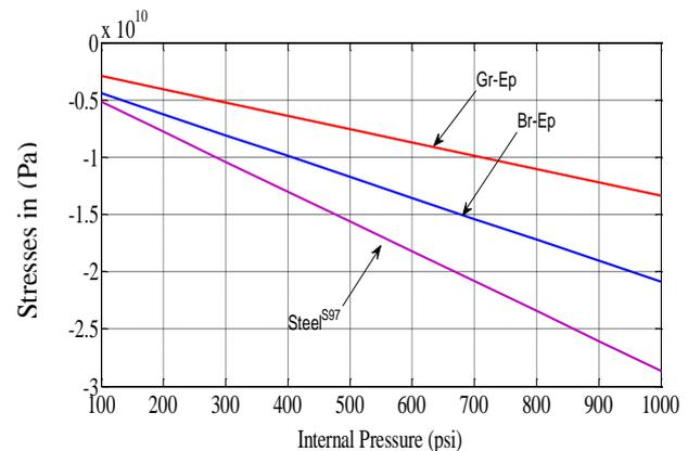
Fig. 4, Buckling stress in pipeline internally pressurized.
