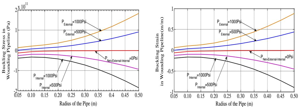
Fig. 5, Buckling stress on the left and strain on the right, that induced into the pipeline during laying installations with and without internally pressurized for Steel<sup>S97</sup>.
