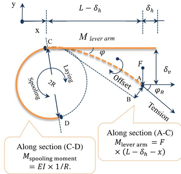
Fig. 2, Schematic of reeling mechanism.
