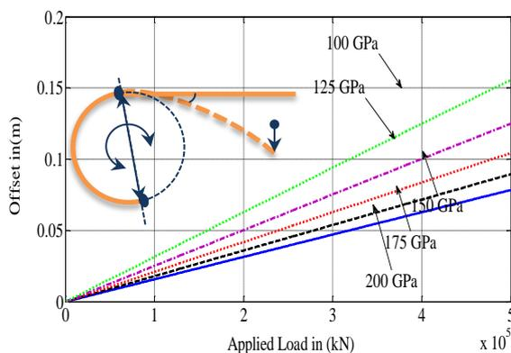
Fig. 3, Simulation shows the plastic deformation of wide range of stiffness that occurs when reeling pipelines of radius equal to 0.15m into drum of dim=6m.
