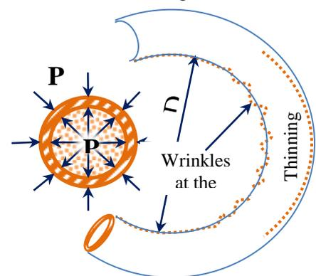
Fig. 1, Ovalization in reeling mechanism due to inward stresses.
