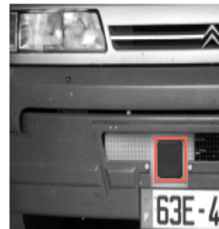
Fig. 1. Radar system mounted on the front end [6]
