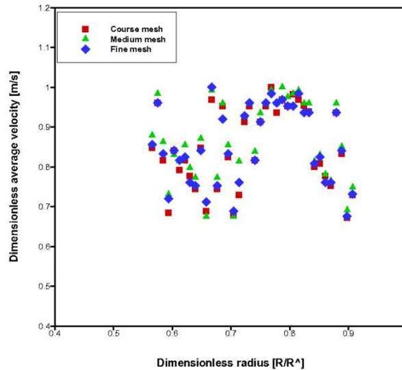
Fig. 2 Quantitative comparison of dimensionless average velocities with various meshes
