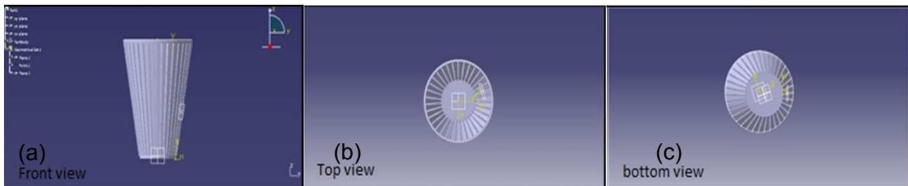
Fig. 1 Geometrical model of perforated rotating bucket in 3D,
