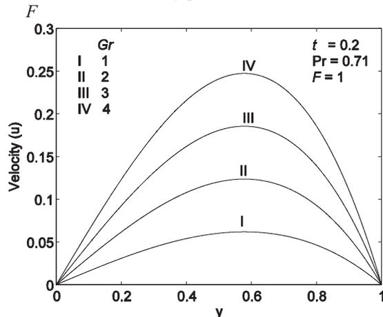
FIGURE 5. Velocity profiles for different  $Gr$
