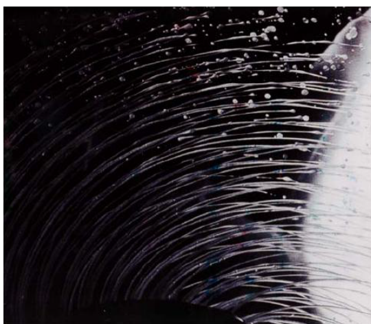
Fig. 1: A top view of the prilling bucket rotating anticlockwise (Wallwork et al. , 2001)
