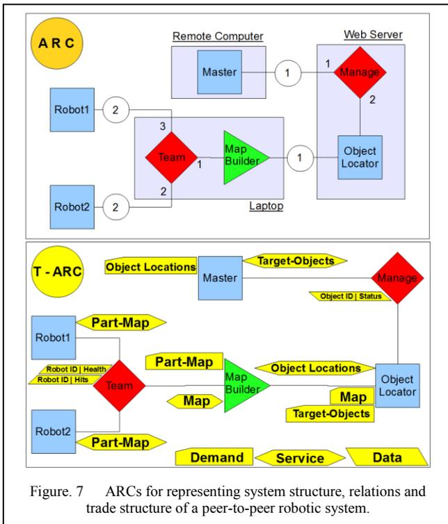
Figure. 7 ARCs for representing system structure, relations and trade structure of a peer-to-peer robotic system.
