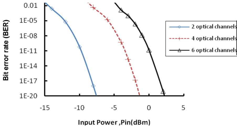
Figure 4. BER against input power simulated with various numbers of optical channels.
