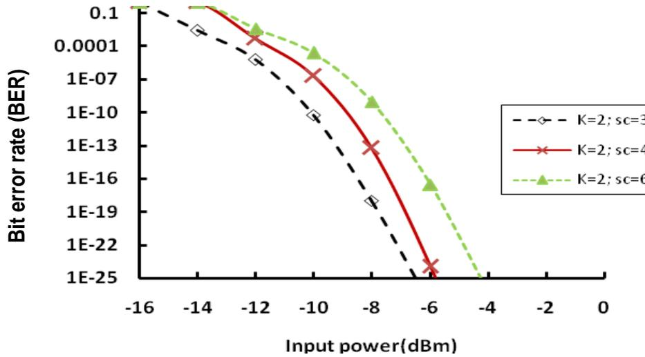
Figure 5. BER against input power simulated with different number of subcarrier channels.
