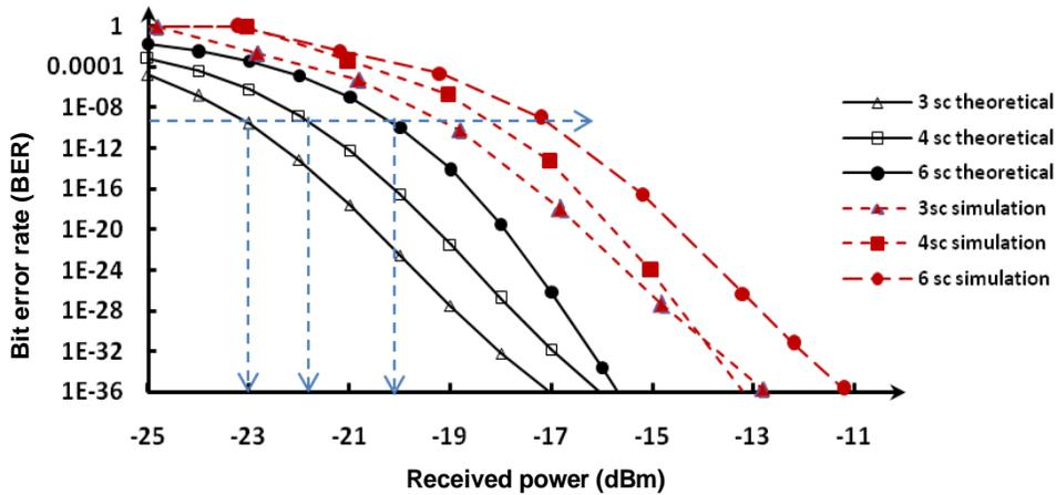
Figure 3. BER against received power with different number of subcarriers for theoretical (black lines) and simulations (red dashes).
