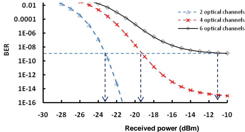
**Figure 2.** Bit error rates (BER) versus received power for the conventional OCDMA network when optical channels are increased from 2, 4 and 6.
