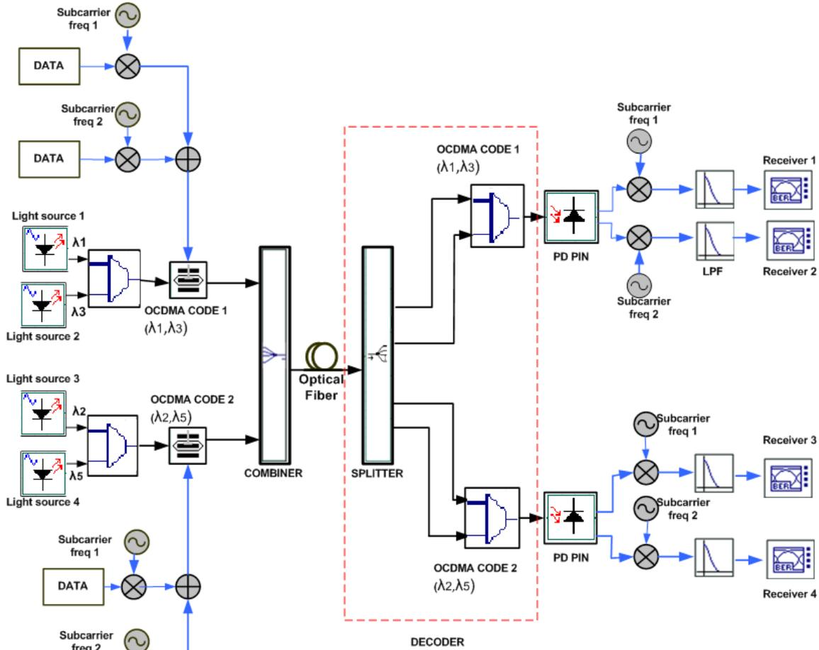
Figure 1. The hybrid SCM/OCDMA system configuration.
