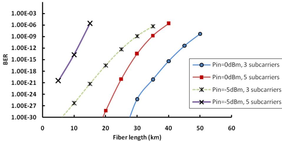
Figure 6. Variation of BER with respect to fiber length for different subcarrier numbers.
