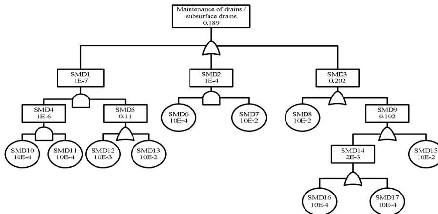
Figure 3: Fault tree logic of maintenance of special measures like surface/subsurface drainage
