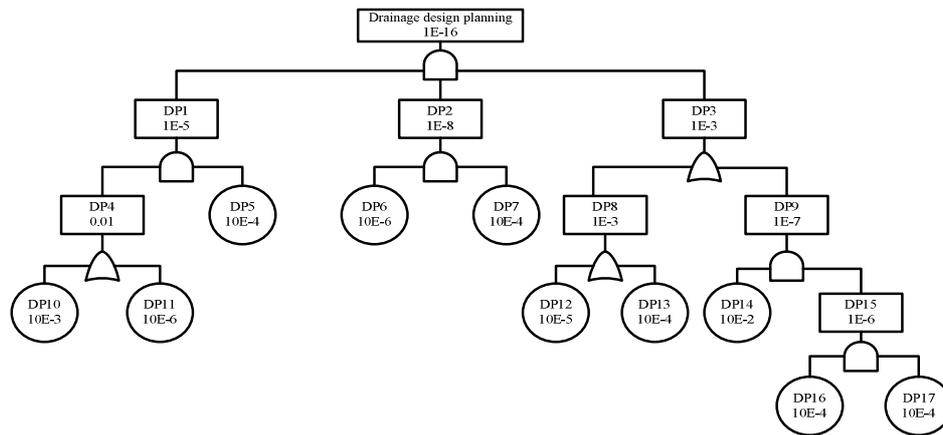
Figure 2: Fault tree logic of drainage design planning
