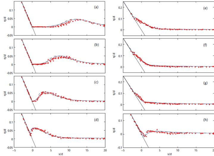
Figure 3 Sequence showing the approach and run-up of a breaking solitary wave. The dots represent laboratory data obtained by Synolakis [22]. The dash line is a nonlinear shallow water solution and the solid line represents numerical results of a Boussinesq model.
