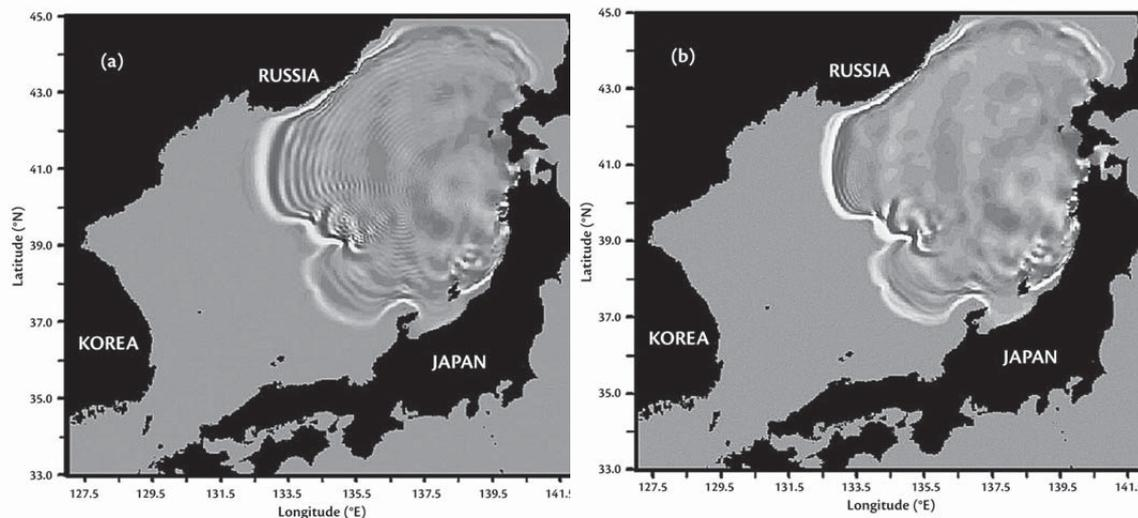
Figure 2 Simulation of Nihonkai-Chubu tsunami of May 26, 1983 in the Japan Sea. Numerical model results from Yoon [26]. Left frame shows simulated wave with dispersive effects included in the numerical model. Right frame shows results without dispersive effects.
