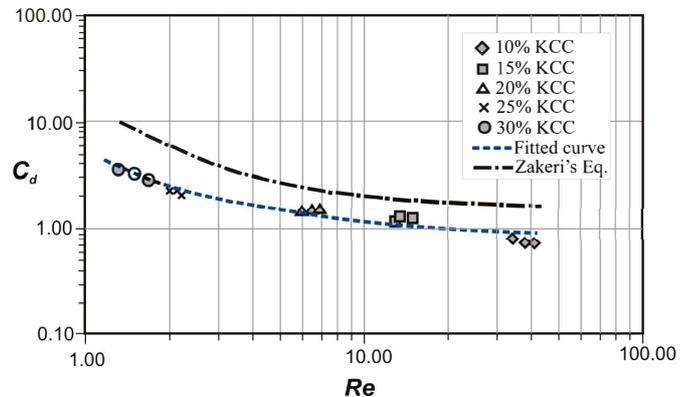
Figure 6. Drag force as relative to Reynolds number for each percentage of KCC, fitted curve, and previous study's formulation
