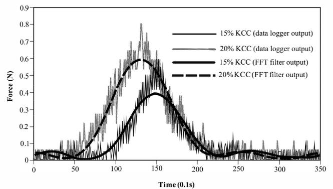
Figure 4. Force responses of data logger output and FFT filtered output of 15% KCC and 20% KCC mudflows on suspended pipe stem (OD 21.3 mm)
