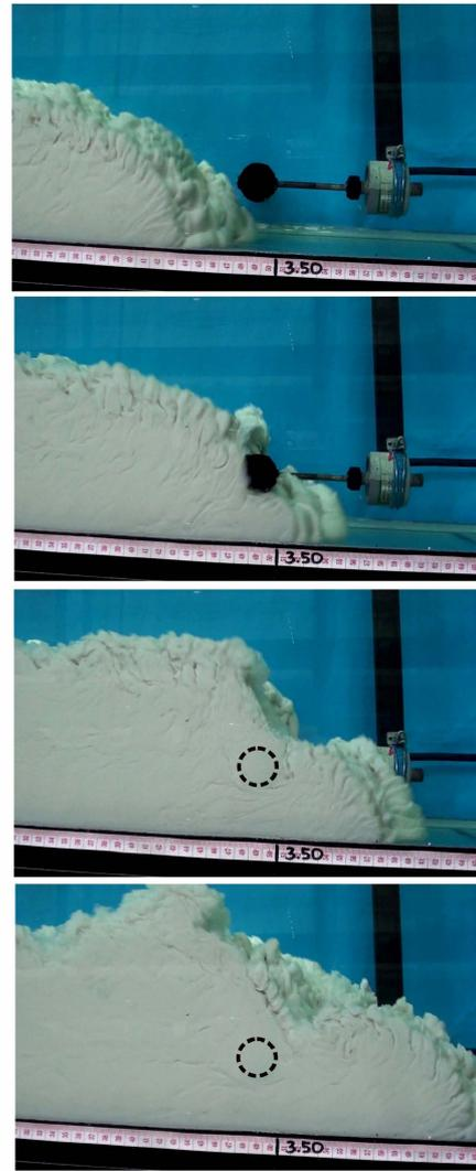
Figure 3. Collision events of 15% KCC mudflows against suspended pipe stem of 21.3 mm OD;  $H/d$  ratio: 18.3;  $u$ : 0.25 m/s. Consecutive captured images are taken within duration of 0.81 s.
