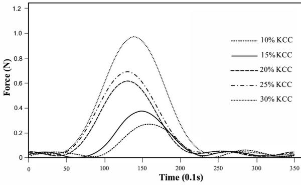
Figure 5. Force responses of FFT filter output of each percentage of KCC (H/d: 18.3)
