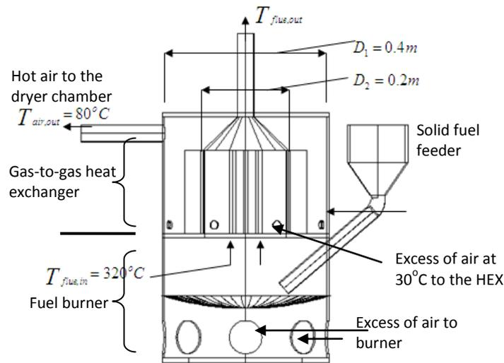
Figure 2: Sketch of the thermal backup unit comprise of slid fuel burner and Gas-to-Gas heat exchanger.
