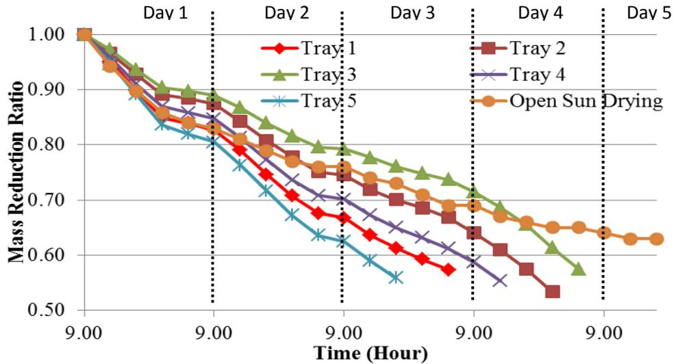
Figure 3: Drying of EFB under solar mode only
