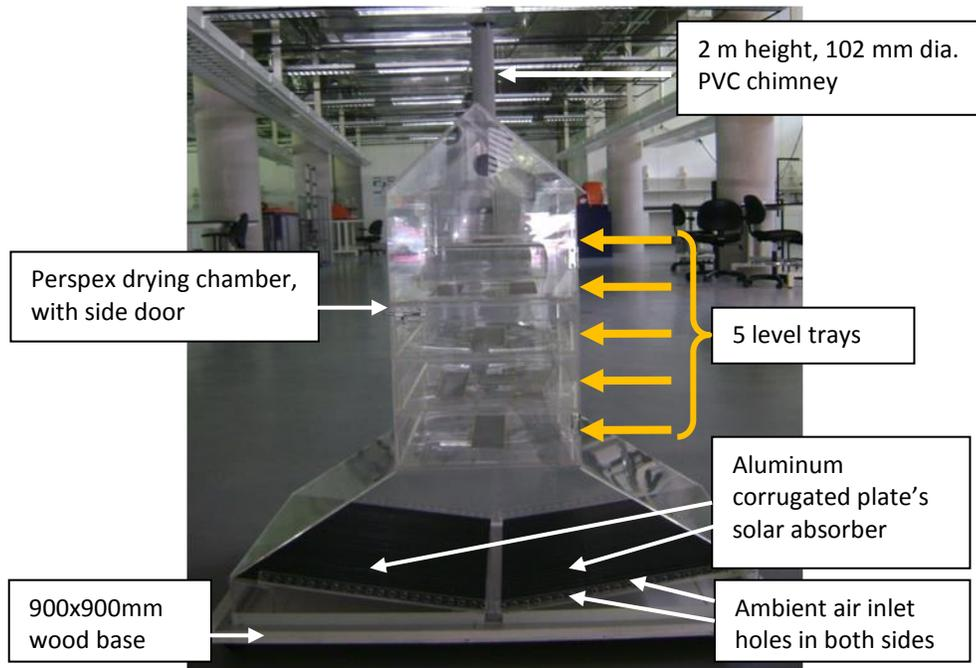
Figure 1: The parameter assumption of solar dryer
