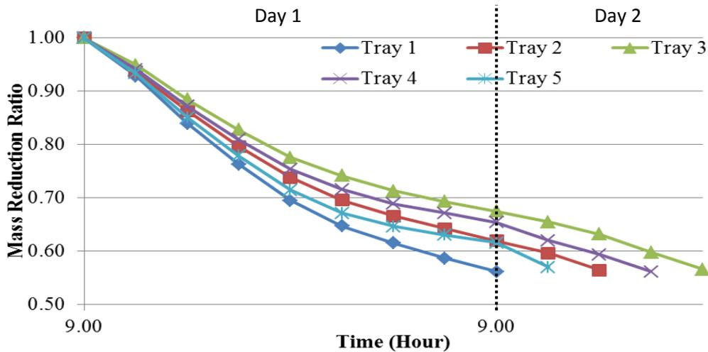
Figure 5: Drying of EFB under hybrid mode
