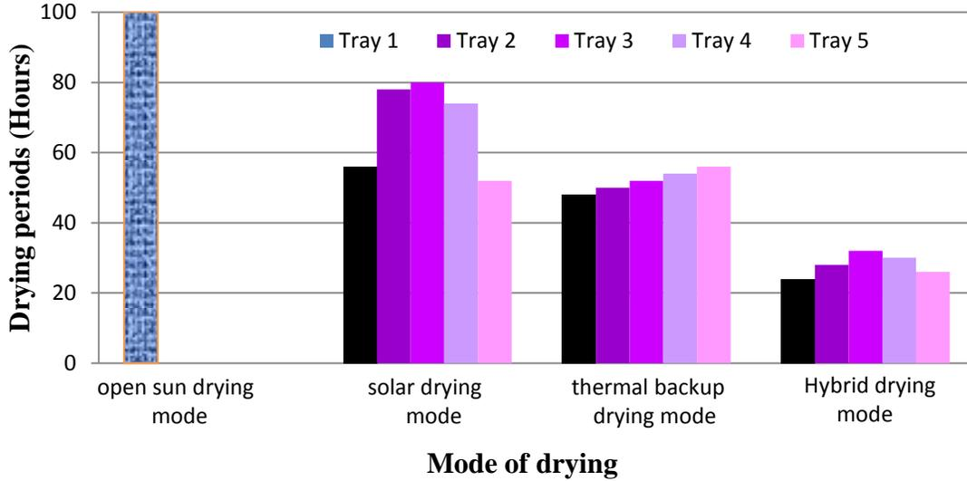
Figure 6: The overall comparison of EFB drying under different modes
