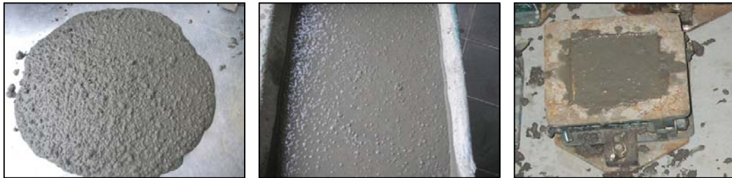
Figure-3. SCC in plastic state - homogeneous, non-segregating and no bleeding.
