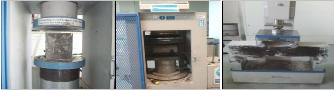
Figure-7. Compressive, splitting tensile and flexural strength tests.
