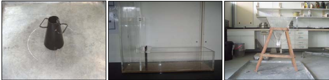
Figure-4. Slump flow, L-box and V-funnel for fresh tests.
