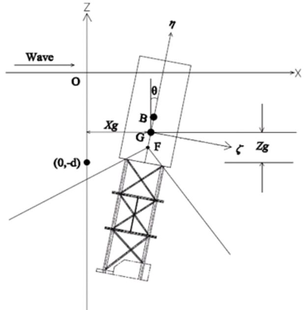
Fig. 4 Three-DOF surge-heave-pitch model of the spar
