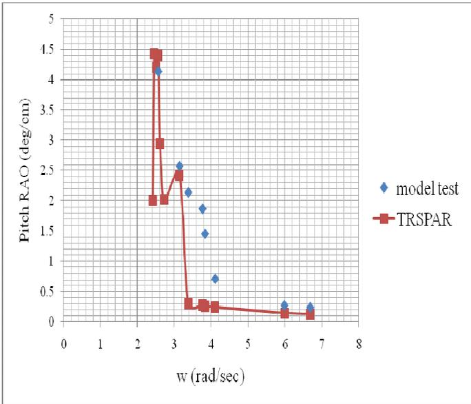
Fig. 7 Comparison of pitch motion RAO
