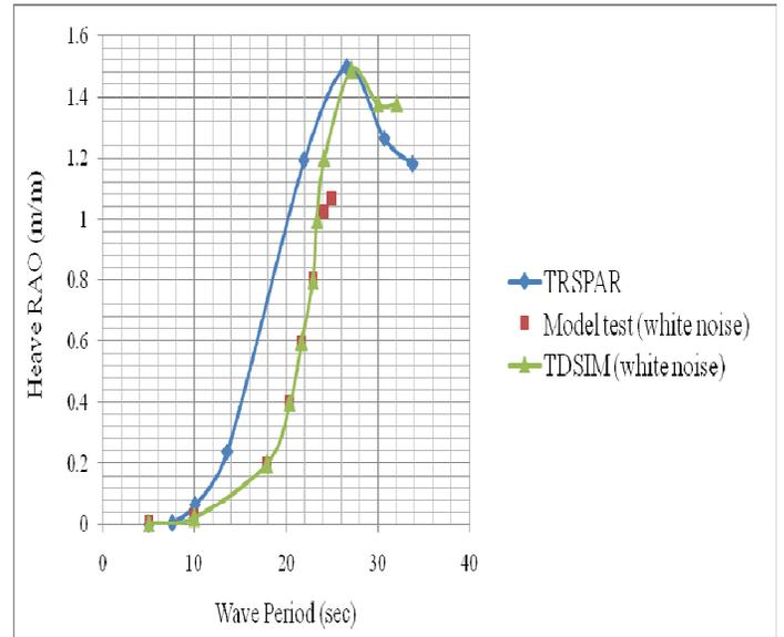
Fig. 9 Comparison of heave RAO at zero degree heading
