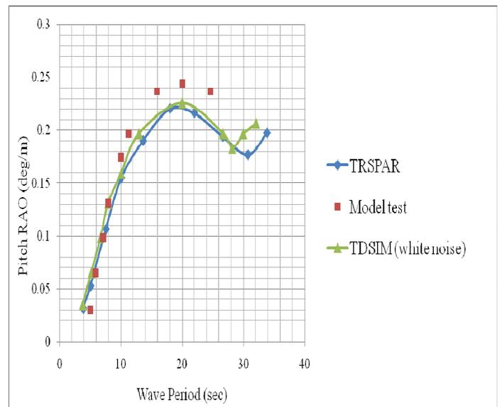
Fig. 10 Comparison of pitch RAO at zero degree heading
