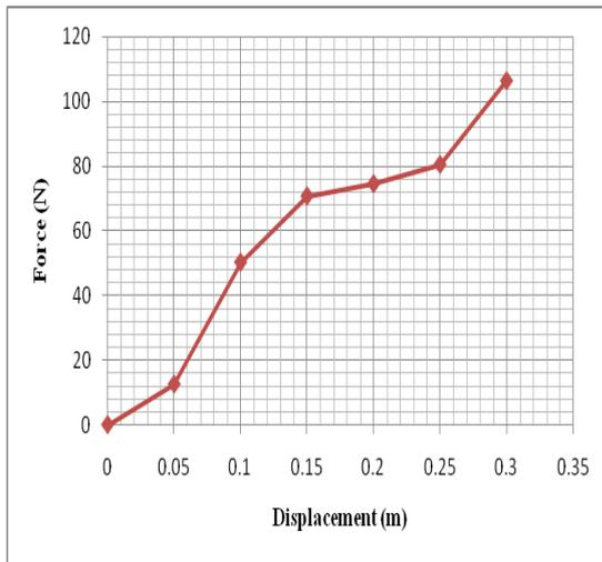
Figure 3 - Force-displacement relationship of the mooring lines
