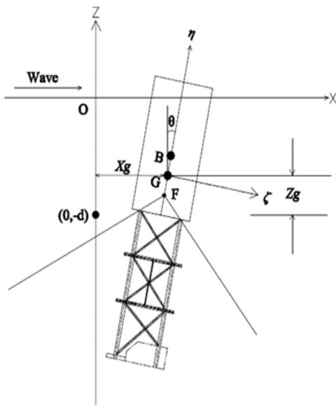
Figure -5 Three-DOF surge-heave-pitch model of the spar
