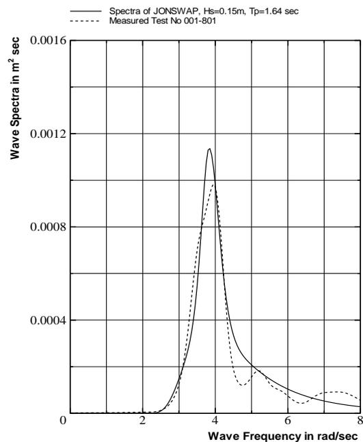
Figure 4 – Comparison between theoretical and measured wave spectrum
