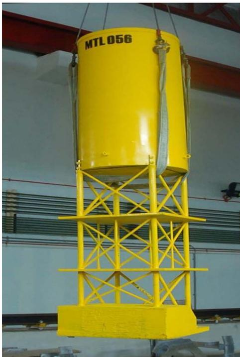
Figure 1 - Truss spar model (Scale: 1:73)
