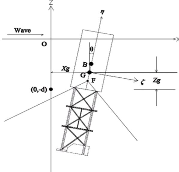
Figure 1: Three degree of freedom surge-heave-pitch model of the spar where:
