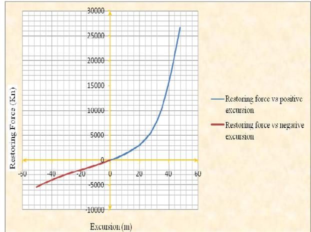
Figure 3: Surge static offset test: offset vs. restoring force.
