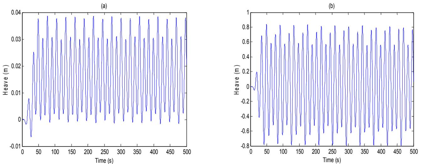
Figure 3. Heave response in regular waves (LC1) (a)Classic spar (b)Truss spar
