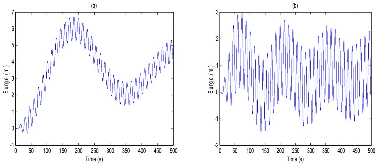
Figure 5. Surge response in regular waves (LC2) (a)Classic spar (b)Truss spar
