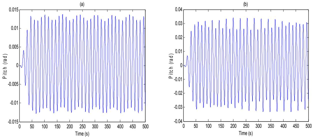
Figure 7. Pitch in regular waves (LC2) (a)Classic spar (b)Truss spar
