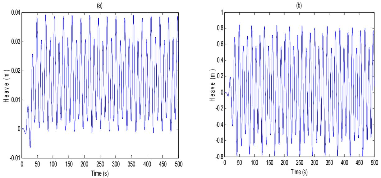
Figure 6. Heave response in regular waves (LC2) (a)Classic spar (b)Truss spar
