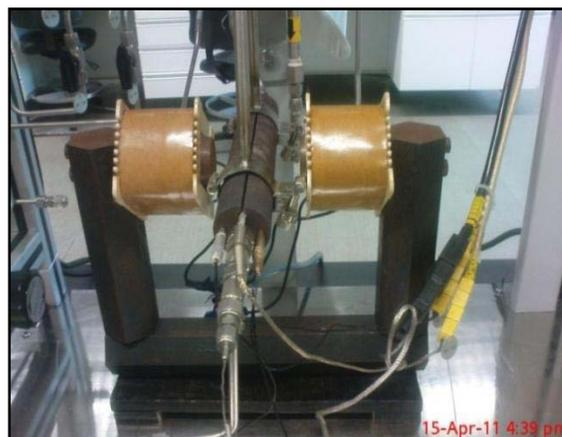
FIGURE 1. Magnetic Induction Reaction Zone
