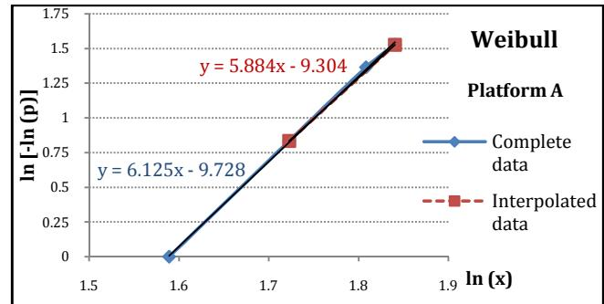
Fig. 2. Data interpolation via Weibull's cumulative distribution function
