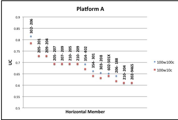
Fig. 4. Comparison of UC for critical horizontal members at different met-ocean combinations
