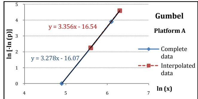
Fig. 3. Data interpolation via Gumbel's cumulative distribution function
