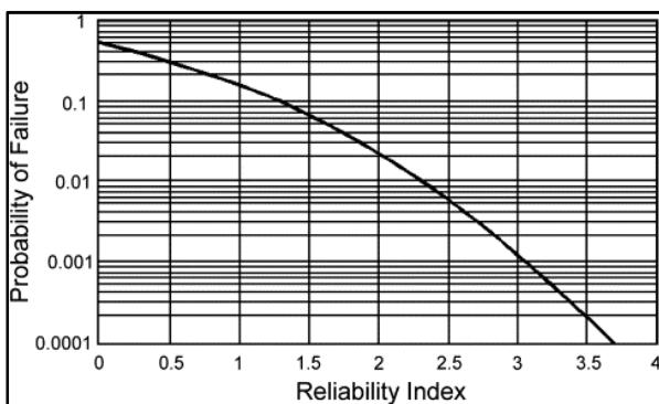
Fig. 6. Relationship between reliability index and probability of failure
