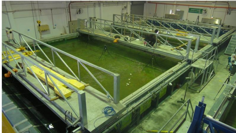
Figure 1 Wave tank equipped with wave generator
